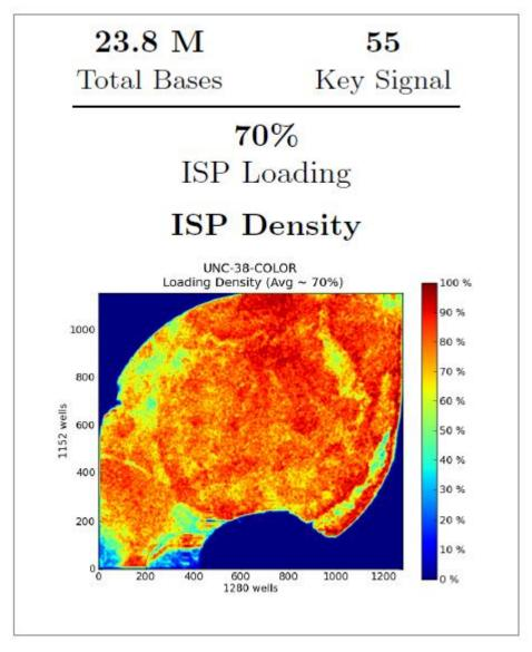
Figure 3.3 : Ion torrent ISP Density
