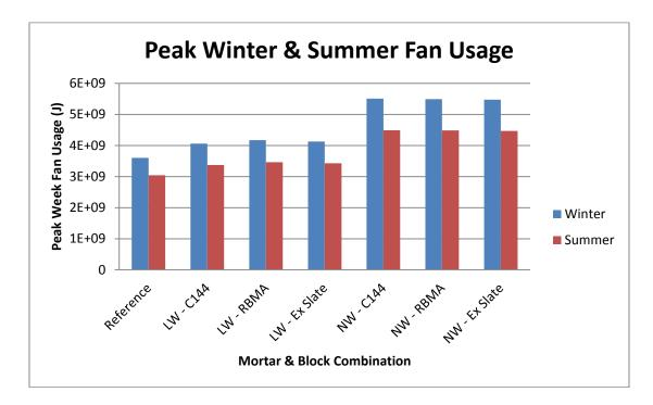
Figure 46: Minneapolis, MN strip mall concrete masonry model fan usage for peak summer and winter times
