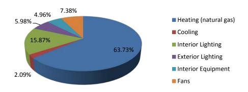
Figure 45: Minneapolis, MN strip mall normal weight concrete masonry model with expanded slate mortar annual energy consumption by end-use
