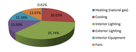
Figure 18: Miami, FL strip mall lightweight concrete masonry model with RBMA mortar annual energy consumption by end-use
