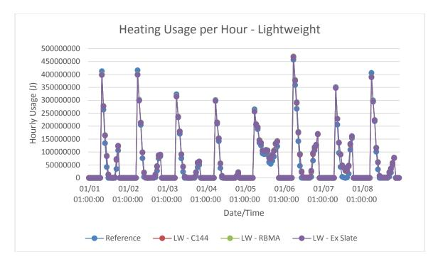
Figure B-9: Los Angeles, CA lightweight models hourly heating energy consumption in winter
