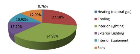
Figure 17: Miami, FL strip mall normal weight C144 concrete masonry model annual energy consumption by end-use
