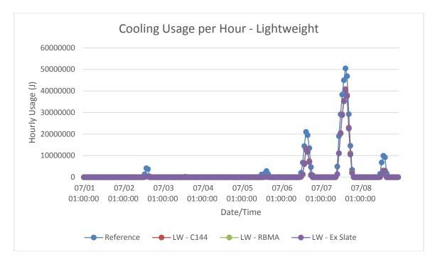
Figure B-25: Seattle, WA lightweight models hourly cooling energy consumption in summer
