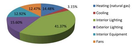
Figure 33: Los Angeles, CA strip mall normal weight C144 concrete masonry model annual energy consumption by end-use
