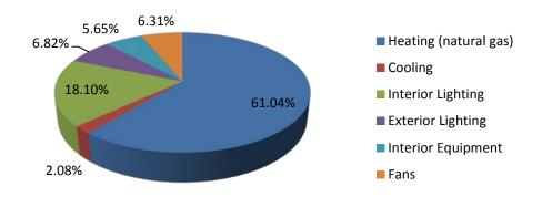
Figure 40: Minneapolis, MN strip mall lightweight C144 concrete masonry model annual energy consumption by end-use
