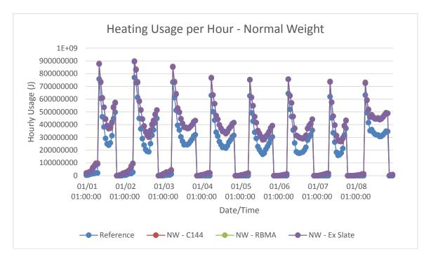
Figure B-24: Seattle, WA normal weight models hourly heating energy consumption in winter
