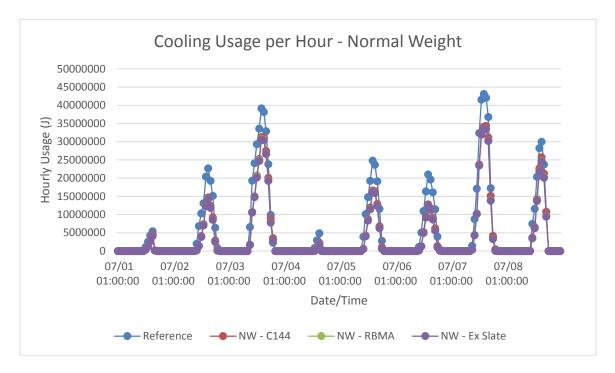
Figure B-12: Los Angeles, CA normal weight models hourly cooling energy consumption in summer
