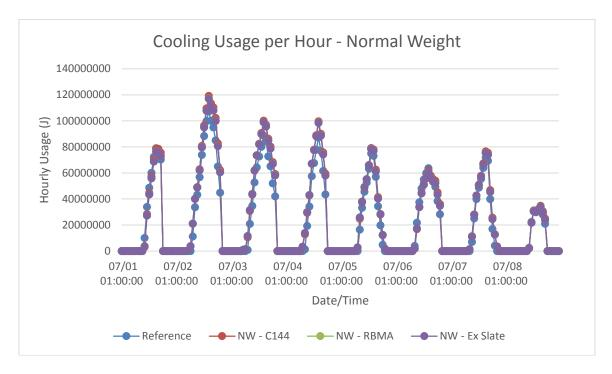
Figure B-8: Boulder, CO normal weight models hourly cooling energy consumption in summer
