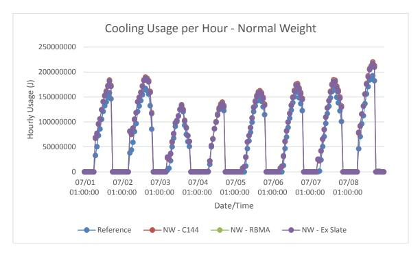
Figure B-22: Phoenix, AZ normal weight models hourly cooling energy consumption in summer
