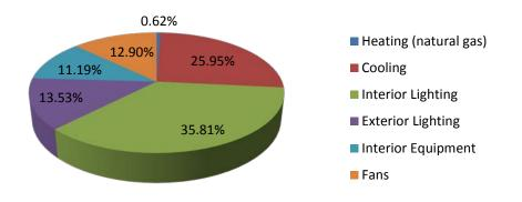
Figure 16: Miami, FL strip mall lightweight C144 concrete masonry model annual energy consumption by end-use
