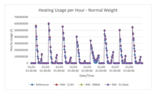
Figure B-20: Phoenix, AZ normal weight models hourly heating energy consumption in winter
