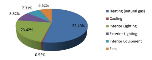
Figure 69: Seattle, WA strip mall normal weight concrete masonry model with expanded slate mortar annual energy consumption by end-use
