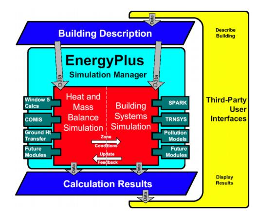
Figure 3: EnergyPlus simulation structure (Crawley et al., 2000)
