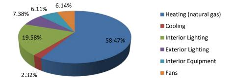
Figure 39: Minneapolis, MN strip mall DOE reference model annual energy consumption by end-use
