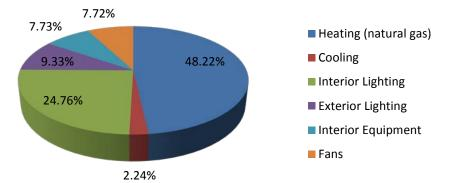
Figure 24: Boulder, CO strip mall lightweight C144 concrete masonry model annual energy consumption by end-use
