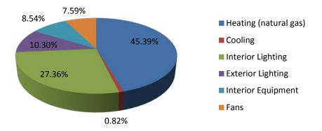
Figure 63: Seattle, WA strip mall DOE reference model annual energy consumption by end-use
