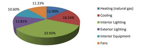
Figure 59: Phoenix, AZ strip mall lightweight concrete masonry model with expanded slate mortar annual energy consumption by end-use
