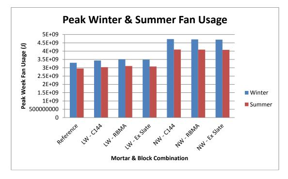
Figure 30: Boulder, CO strip mall concrete masonry model fan usage for peak summer and winter times
