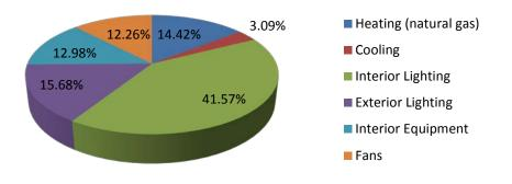
Figure 36: Los Angeles, CA strip mall normal weight concrete masonry model with RBMA mortar annual energy consumption by end-use
