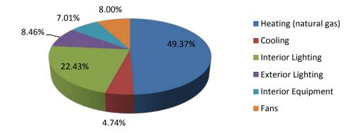
Figure 52: Baltimore, MD strip mall normal weight concrete masonry model with RBMA mortar annual energy consumption by end-use
