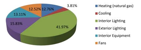
Figure 31: Los Angeles, CA strip mall DOE reference model annual energy consumption by end-use
