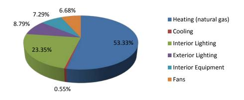
Figure 65: Seattle, WA strip mall normal weight C144 concrete masonry model annual energy consumption by end-use
