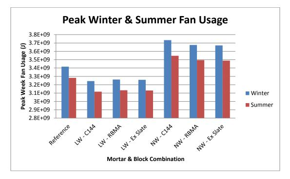
Figure 54: Baltimore, MD strip mall concrete masonry model fan usage for peak summer and winter times
