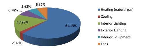
Figure 43: Minneapolis, MN strip mall lightweight concrete masonry model with expanded slate mortar annual energy consumption by end-use
