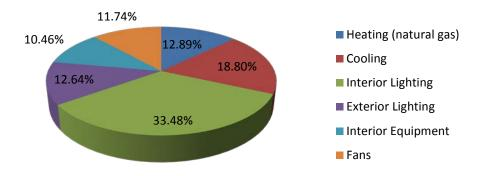
Figure 55: Phoenix, AZ strip mall DOE reference model annual energy consumption by end-use
