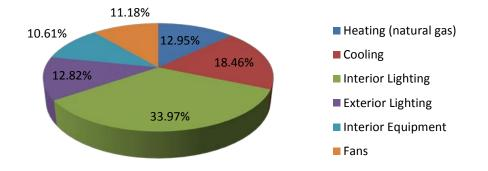
Figure 56: Phoenix, AZ strip mall lightweight C144 concrete masonry model annual energy consumption by end-use
