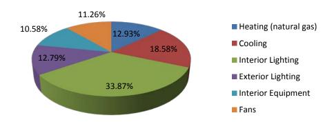
Figure 58: Phoenix, AZ strip mall lightweight concrete masonry model with RBMA mortar annual energy consumption by end-use
