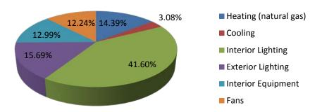
Figure 37: Los Angeles, CA strip mall normal weight concrete masonry model with expanded slate mortar annual energy consumption by end-use
