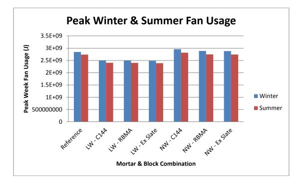
Figure 70: Seattle, WA strip mall concrete masonry model fan usage for peak summer and winter times
