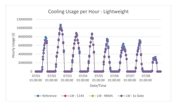
Figure B-7: Boulder, CO lightweight models hourly cooling energy consumption in summer
