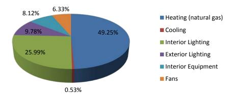
Figure 66: Seattle, WA strip mall lightweight concrete masonry model with RBMA mortar annual energy consumption by end-use
