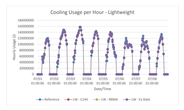
Figure B-3: Miami, FL lightweight models hourly cooling energy consumption in summer
