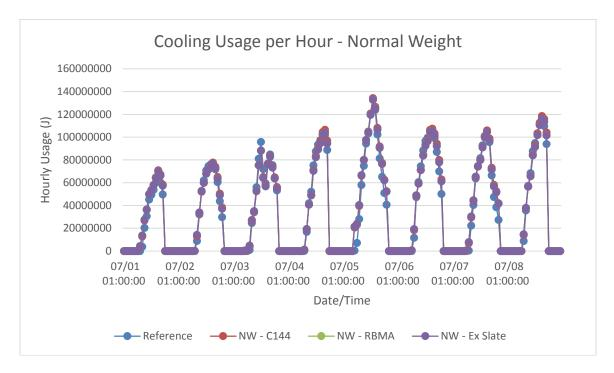
Figure B-18: Baltimore, MD normal weight models hourly cooling energy consumption in summer
