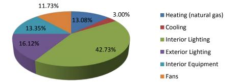
Figure 35: Los Angeles, CA strip mall lightweight concrete masonry model with expanded slate mortar annual energy consumption by end-use
