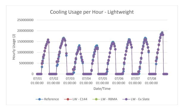
Figure B-21: Phoenix, AZ lightweight models hourly cooling energy consumption in summer
