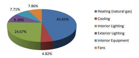
Figure 50: Baltimore, MD strip mall lightweight concrete masonry model with RBMA mortar annual energy consumption by end-use
