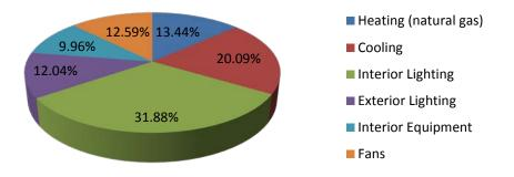
Figure 57: Phoenix, AZ strip mall normal weight C144 concrete masonry model annual energy consumption by end-use
