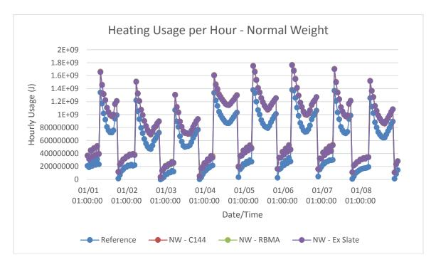
Figure B-14: Minneapolis, MN normal weight models hourly heating energy consumption in winter
