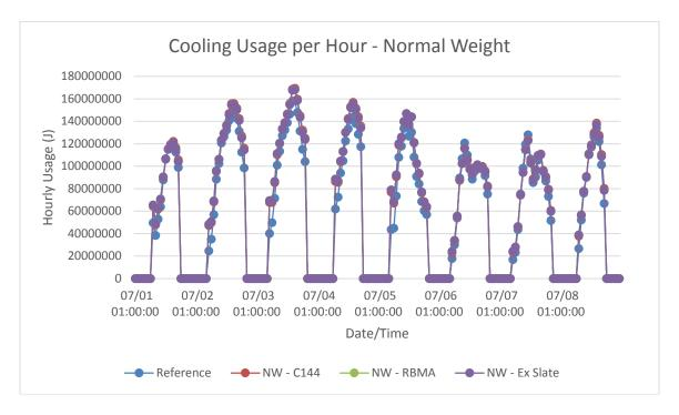
Figure B-4: Miami, FL normal weight models hourly cooling energy consumption in summer
