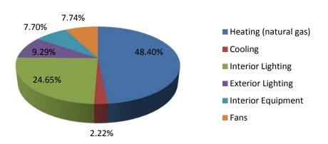
Figure 27: Boulder, CO strip mall lightweight concrete masonry model with expanded slate mortar annual energy consumption by end-use
