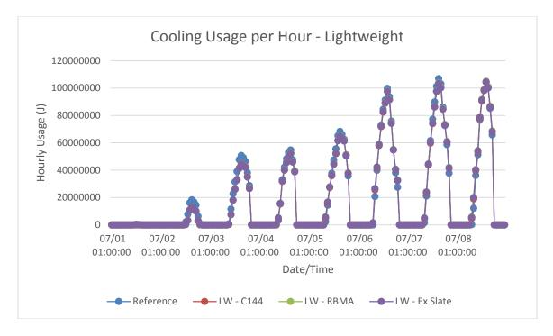
Figure B-14: Minneapolis, MN lightweight models hourly cooling energy consumption in summer
