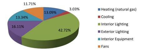
Figure 32: Los Angeles, CA strip mall lightweight C144 concrete masonry model annual energy consumption by end-use
