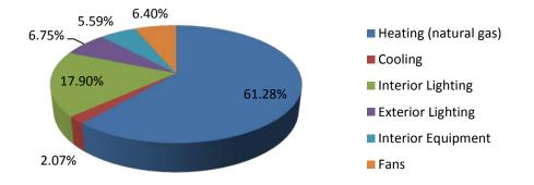
Figure 42: Minneapolis, MN strip mall lightweight concrete masonry model with RBMA mortar annual energy consumption by end-use
