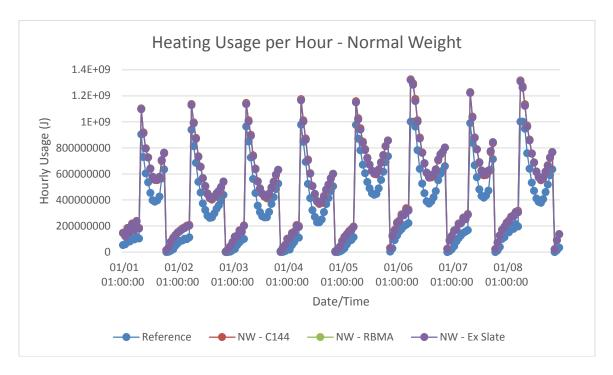
Figure B-6: Boulder, CO normal weight models hourly heating energy consumption in winter
