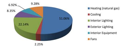
Figure 28: Boulder, CO strip mall normal weight concrete masonry model with RBMA mortar annual energy consumption by end-use
