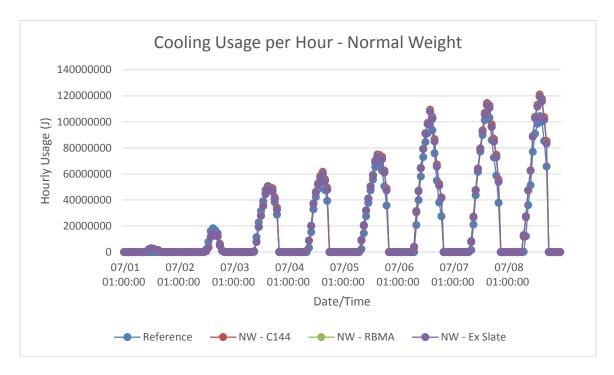
Figure B-14: Minneapolis, MN normal weight models hourly cooling energy consumption in summer
