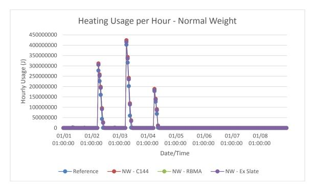
Figure B-2: Miami, FL normal weight models hourly heating energy consumption in winter
