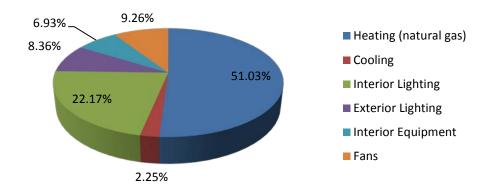
Figure 29: Boulder, CO strip mall normal weight concrete masonry model with expanded slate mortar annual energy consumption by end-use
