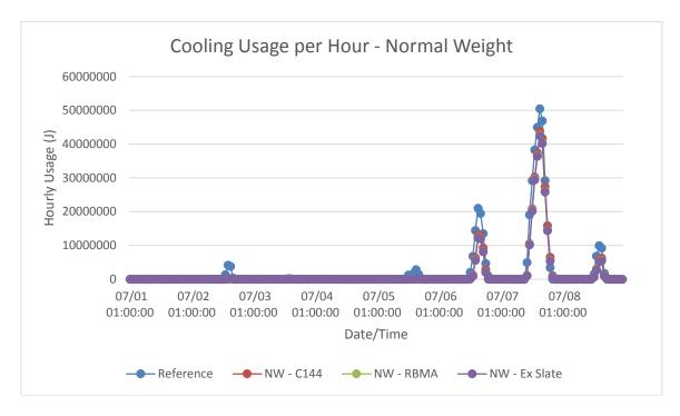
Figure B-26: Seattle, WA normal weight models hourly cooling energy consumption in summer
