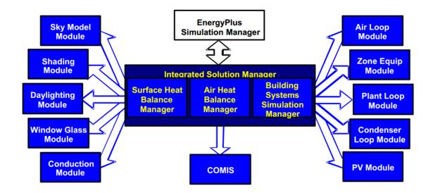
Figure 4: EnergyPlus simulation manager (Crawley et al., 2000)
