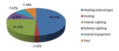
Figure 26: Boulder, CO strip mall lightweight concrete masonry model with RBMA mortar annual energy consumption by end-use
