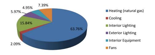
Figure 44: Minneapolis, MN strip mall normal weight concrete masonry model with RBMA mortar annual energy consumption by end-use
