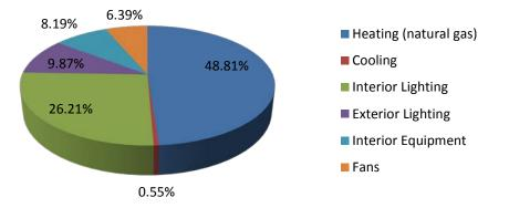
Figure 64: Seattle, WA strip mall lightweight C144 concrete masonry model annual energy consumption by end-use
