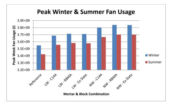
Figure 22: Miami, FL strip mall concrete masonry fan usage for peak summer and winter times
