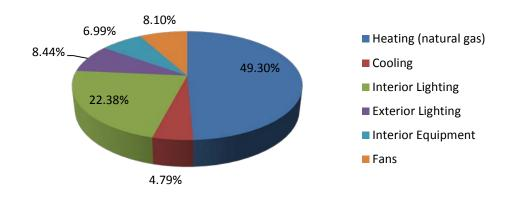
Figure 49: Baltimore, MD strip mall normal weight C144 concrete masonry model annual energy consumption by end-use
