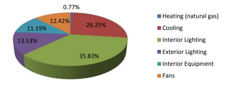
Figure 15: Miami, FL strip mall DOE reference model annual energy consumption by end-use
