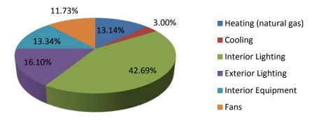
Figure 34: Los Angeles, CA strip mall lightweight concrete masonry model with RBMA mortar annual energy consumption by end-use
