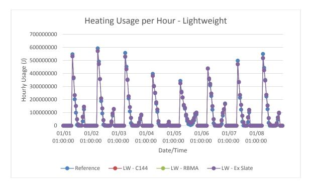
Figure B-19: Phoenix, AZ lightweight models hourly heating energy consumption in winter
