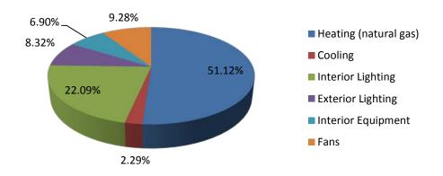
Figure 25: Boulder, CO strip mall normal weight C144 concrete masonry model annual energy consumption by end-use
