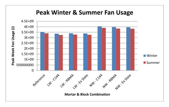
Figure 62: Phoenix, AZ strip mall concrete masonry model fan usage for peak summer and winter times
