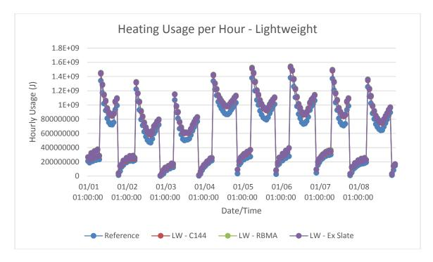
Figure B-13: Minneapolis, MN lightweight models hourly heating energy consumption in winter
