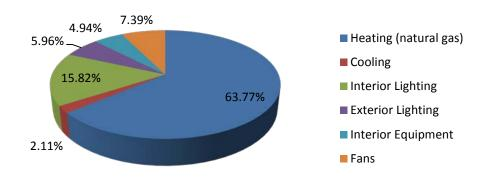
Figure 41: Minneapolis, MN strip mall normal weight C144 concrete masonry model annual energy consumption by end-use
