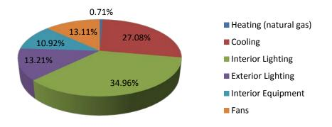
Figure 21: Miami, FL strip mall normal weight concrete masonry model with expanded slate mortar annual energy consumption by end-use
