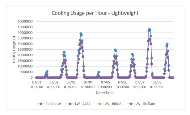
Figure B-11: Los Angeles, CA lightweight models hourly cooling energy consumption in summer
