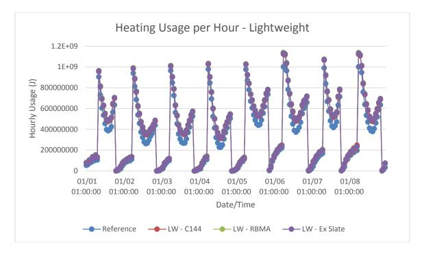
Figure B-5: Boulder, CO lightweight models hourly heating energy consumption in winter
