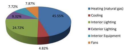
Figure 51: Baltimore, MD strip mall lightweight concrete masonry model with expanded slate mortar annual energy consumption by end-use
