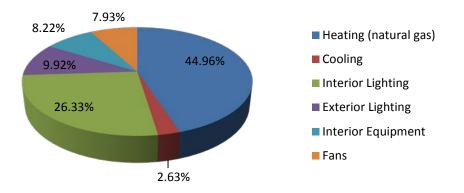
Figure 23: Boulder, CO strip mall DOE reference model annual energy consumption by end-use
