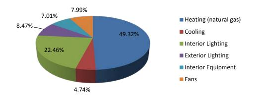
Figure 53: Baltimore, MD strip mall normal weight concrete masonry model with expanded slate mortar annual energy consumption by end-use
