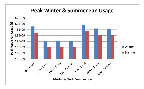
Figure 38: Los Angeles, CA strip mall concrete masonry model fan usage for peak summer and winter times
