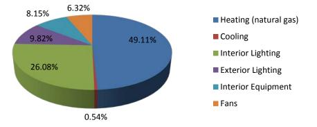
Figure 67: Seattle, WA strip mall lightweight concrete masonry model with expanded slate mortar annual energy consumption by end-use
