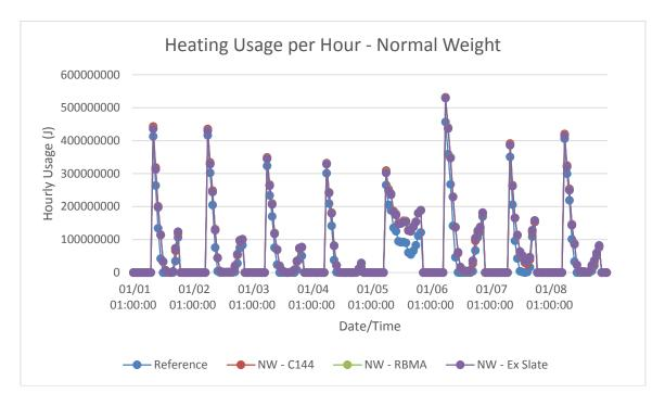
Figure B-10: Los Angeles, CA normal weight models hourly heating energy consumption in winter
