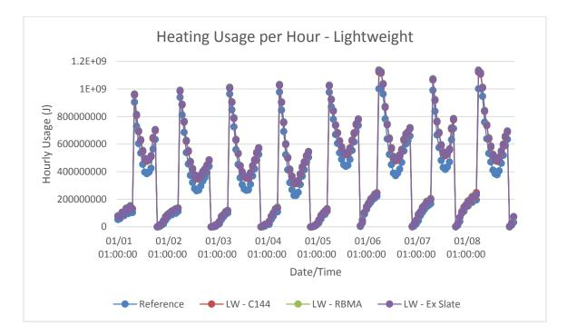
Figure 14: Boulder, CO heating usage per hour for lightweight concrete masonry models example graph
