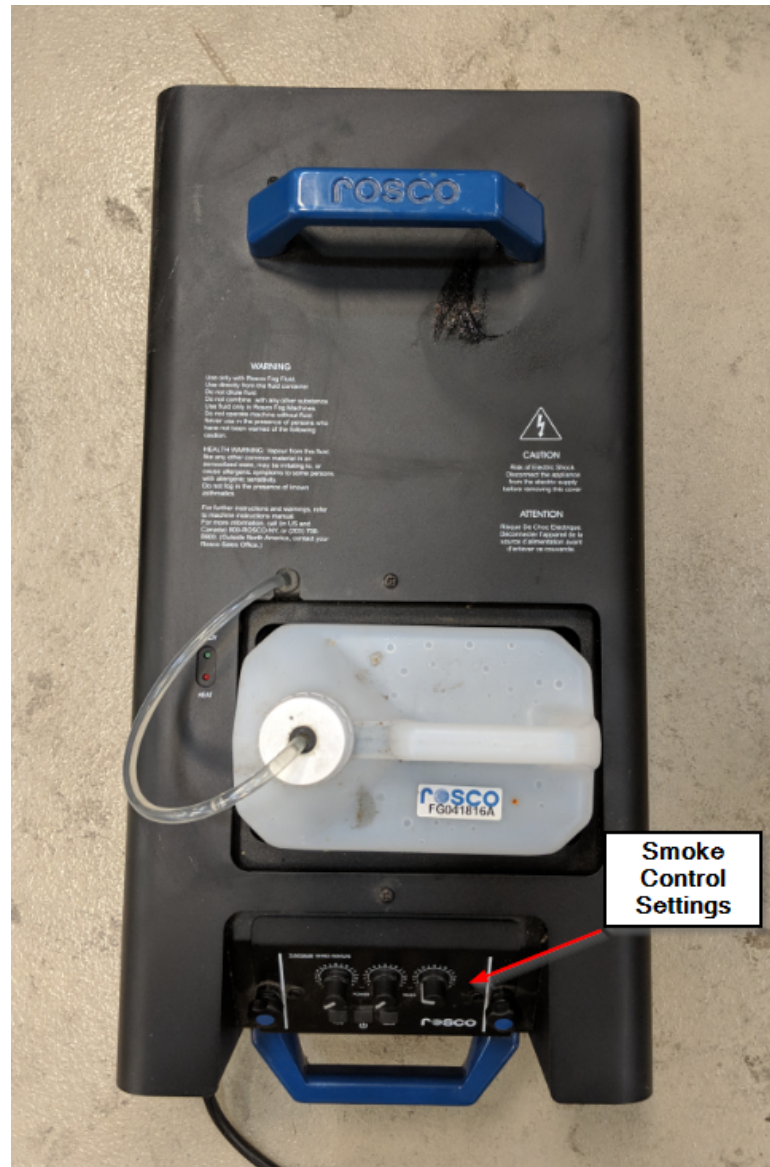
Figure 3.9: Smoke generator used for experimentation
