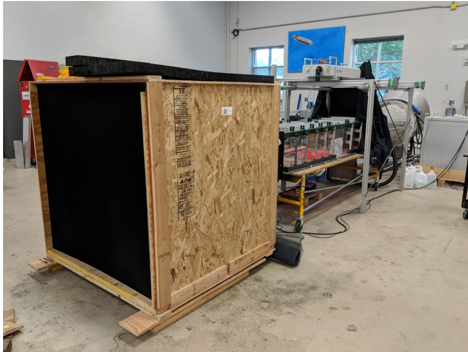
Figure 3.2: Wind tunnel with settling chamber
