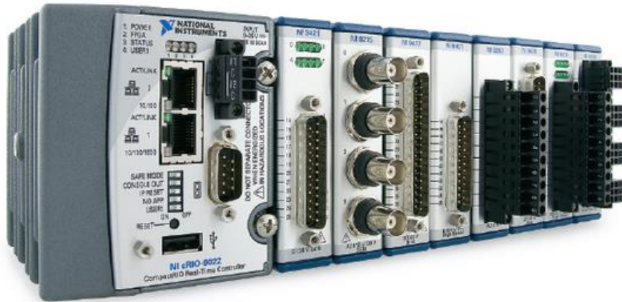
Figure 5: cRIO with different modules for variety of application
