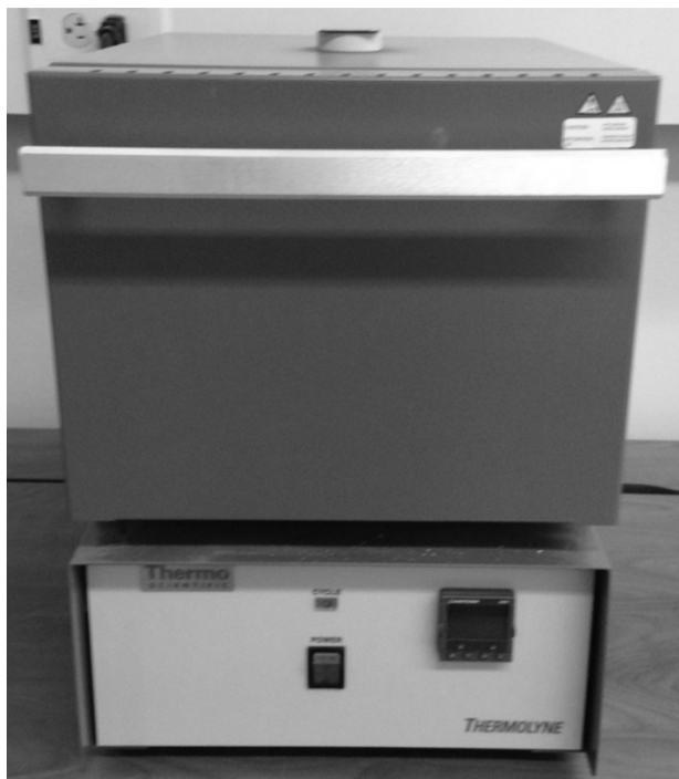
Figure 3: Thermo Scientific furnace used to synthesize quartz and dope Cris
