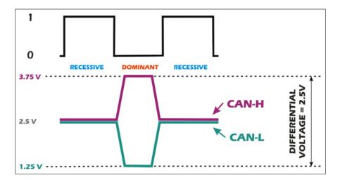
Figure 3.15: CAN Bus Differential Signal Illustration [79]
