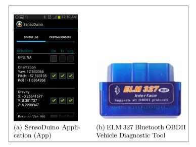
Figure 2.11: SensoDuino App and ELM327 Bluetooth Adapter [24]
