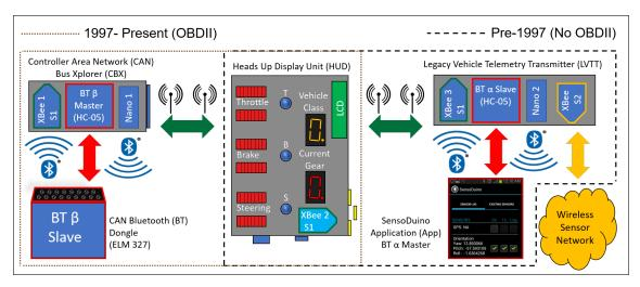
Figure 5.1: High Level Block Diagram
