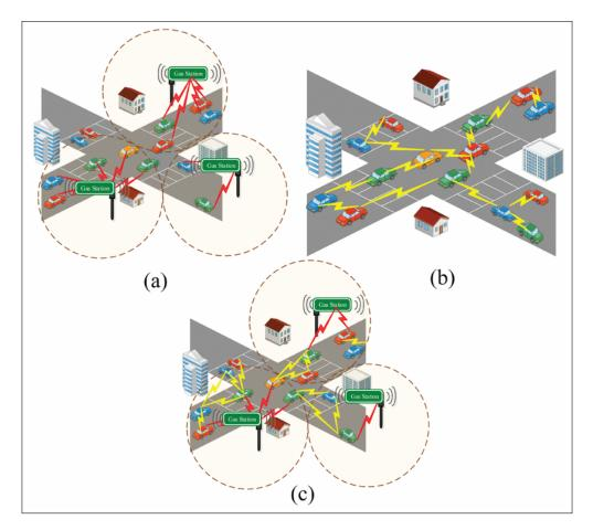
Figure 2.8: The Communication Architecture of VANETs: (a) WAVE Based Wi-Fi; (b) Adhoc; (c) Hybrid [15]
