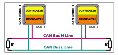
Figure 3.16: CAN Bus Node Components [79]
