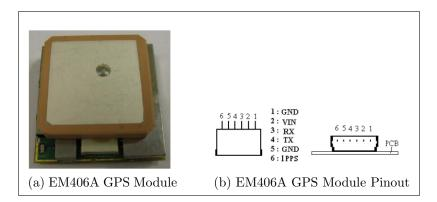
Figure 5.24: EM406A GPS Module and Pinout [100]
