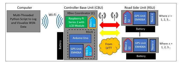
Figure 5.22: WSN High Level Block Diagram
