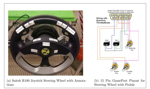
Figure 5.5: Joystick Steering Wheel and Companion Pinout [95]
