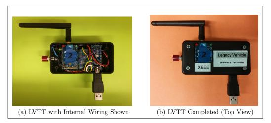
Figure 5.15: LVTT Internal Wiring and Completed Assembly
