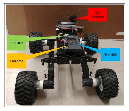
Figure 6.2: Annotated Rover Test Vehicle
