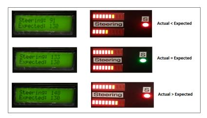
Figure 5.17: HUD Steering Expected Value (Class 3 Vehicle)
