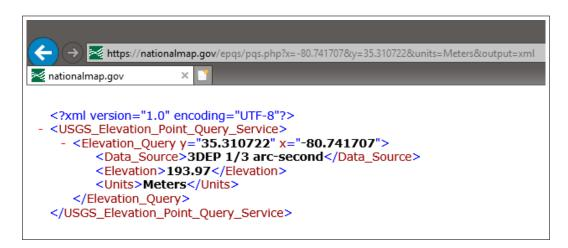
Figure 5.34: USGS Elevation Query Service XML Output [103]
