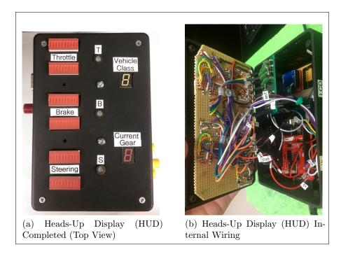
Figure 5.6: Heads-Up Display (HUD) Internal and Complete Assembly
