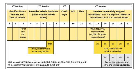
Figure 3.12: Breakdown of NHTSA Required Vehicle VIN Number [77]
