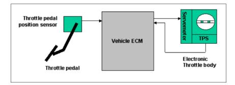
Figure 3.5: Throttle-by-Wire System Block Diagram [67]
