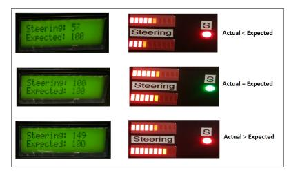
Figure 5.16: HUD Steering Expected Value (Class 2 Vehicle)
