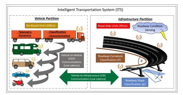
Figure 4.1: Components of an Intelligent Transportation System (ITS) [69, 92]
