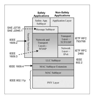
Figure 2.4: Layered Architecture for DSRC Communication [9]
