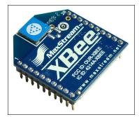
Figure 3.25: XBee S1 Radio Module [90]
