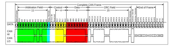
Figure 3.17: CAN Bus Base Frame Format (Without Bit Stuffing) [80]
