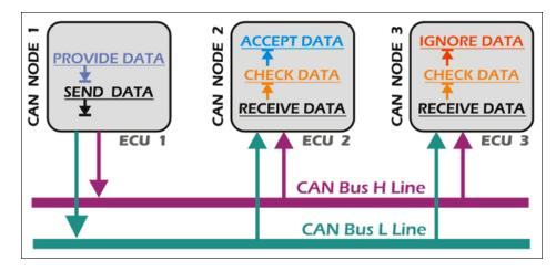
Figure 3.18: CAN Bus General Data Flow Process [79]
