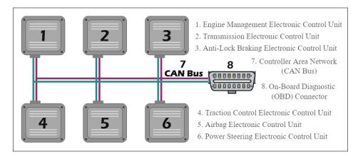
Figure 3.14: Example CAN Bus System Diagram [79]
