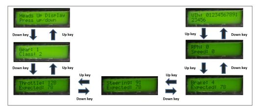
Figure 5.19: Heads-Up Display (HUD) LCD Scroll Menu
