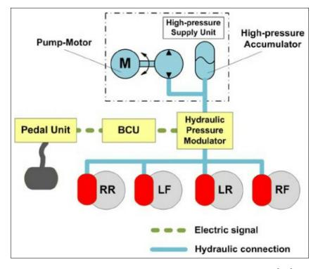
Figure 3.3: Components of a Brake-by-Wire System [65]
