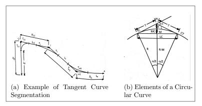
Figure 3.7: Example of Tangent and Circular Curves [74]
