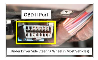
Figure 3.20: OBDII Port (On All Vehicles Produced after 1996) [82]
