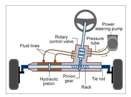
Figure 3.1: Components of a Rack-and-Pinion Steering System [56]
