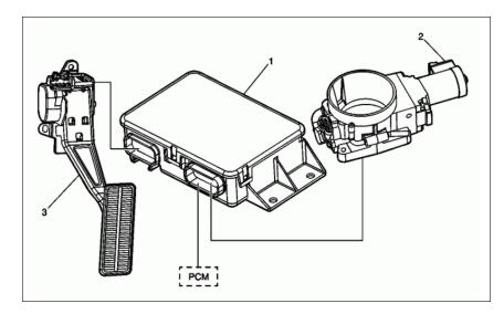
Figure 3.4: Components of a Throttle-by-Wire System [68]
