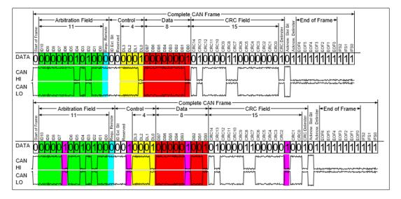
Figure 3.19: CAN Bus Base Frame Format (With Bit Stuffing) [80]
