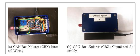
Figure 5.4: CAN Bus Xplorer (CBX) Internal Wiring and Completed Assembly
