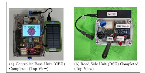
Figure 5.23: CBU and RSU Completed (Top View)
