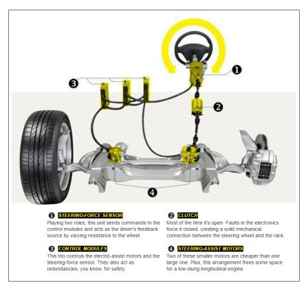
Figure 3.2: Components of a Steering-by-Wire System [57]
