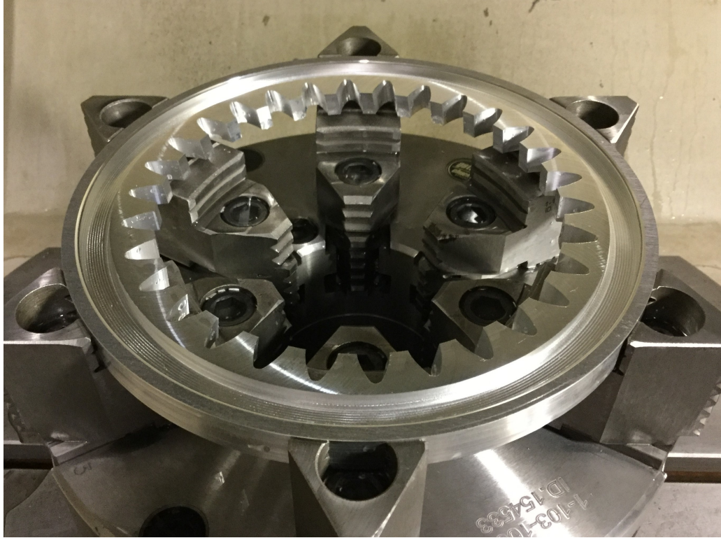
Figure 5.4: Machined Internal Helical Gear with 10^\circ Helix Angle
