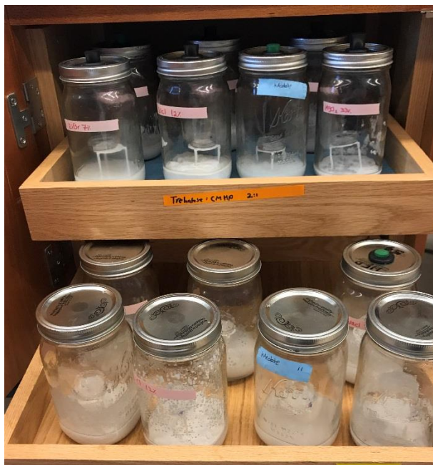
Figure 13. Constant relative humidity jars, using different saturated salt solutions in mason jars
