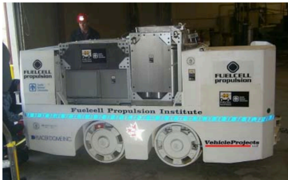
FIGURE 6: Hydrogen fuel cell mining locomotive (Miller & Barnes, 2002)
