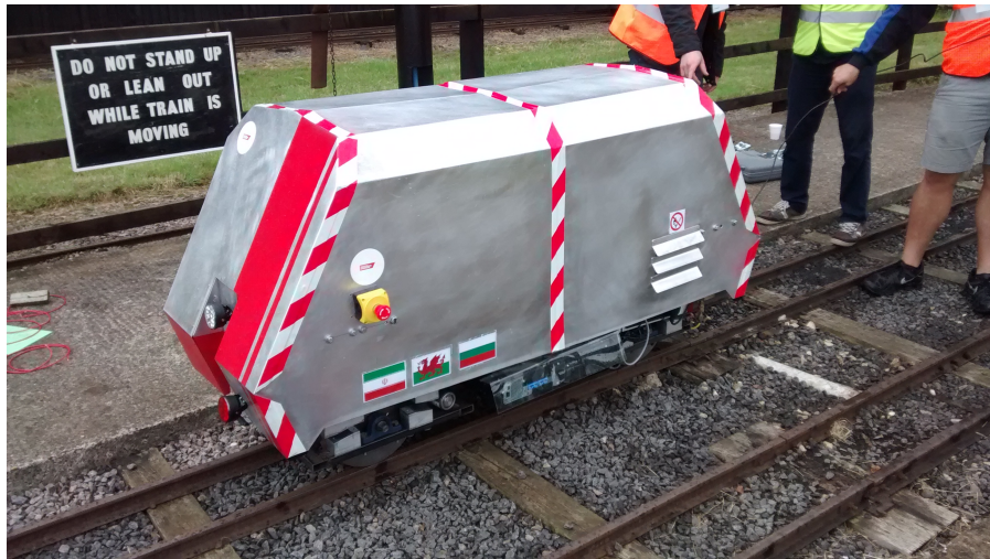
FIGURE 10: 2014 University of Birmingham hydrogen-hybrid locomotive (Author's Collection)
