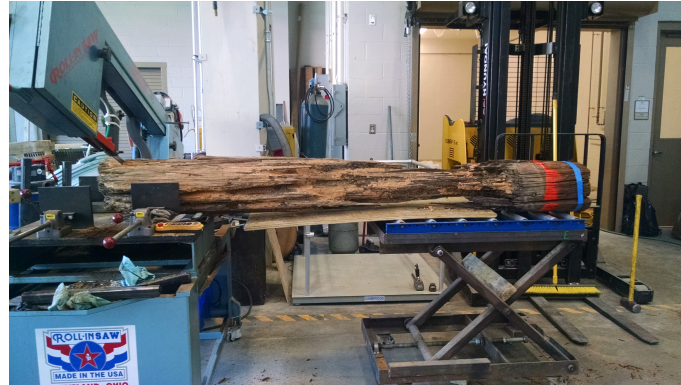
FIGURE 3.12: Destructive characterization of Pole 8 with band saw
