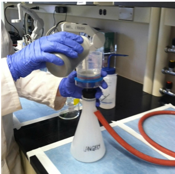
Figure 3: Batch filtration set-up
