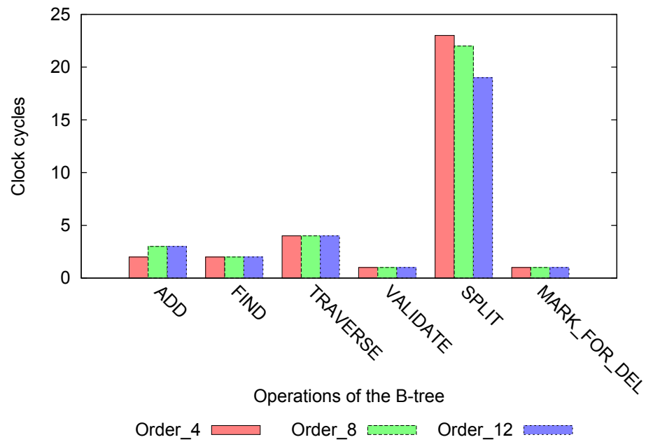
Figure 4.7: Latencies of the operations of the B-tree
