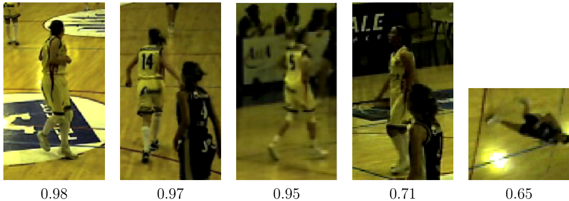
Figure 9: The estimated detection accuracy (Equation 8) for selected image patches. The first patch depicts an ideal case (unoccluded, upright, and near-field). The remaining patches show examples of slight occlusion, smaller height, moderate occlusion, and non-verticality, respectively.
