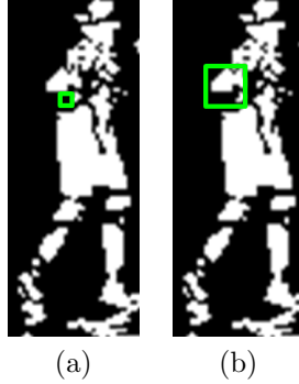
Figure 5: (a) Point sampling takes the single pixel in the image corresponding to the projected voxel center, while (b) area sampling considers the 2D bounding box of the projected voxel’s 3D extent.
