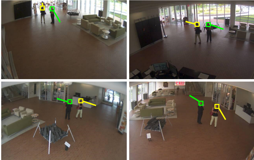
Figure 23: In multi-camera networks, head pose estimation can support applications in surveillance, marketing and HCI. Our method uses an ensemble of exemplars to provide finer-grained predictions than previous approaches.
