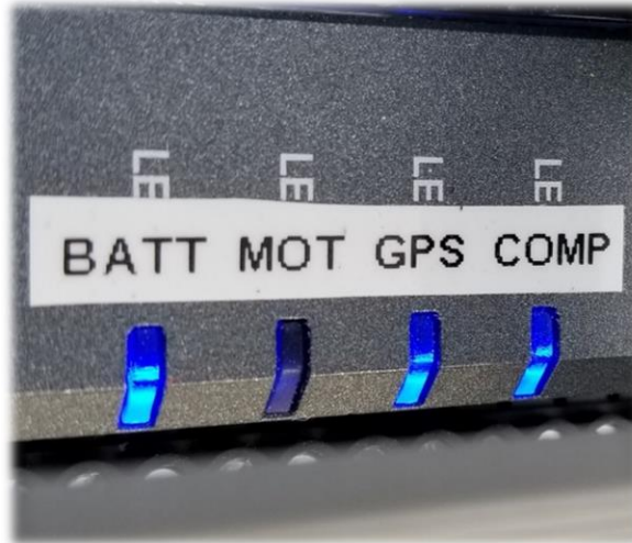
Figure 17: LED indicators on the myRIO controller
