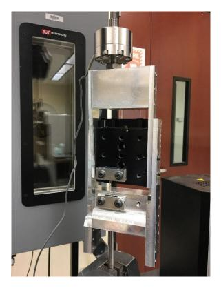
Figure 2.4: Home-built stretching device installed in an Instron uniaxial tensile machine.
