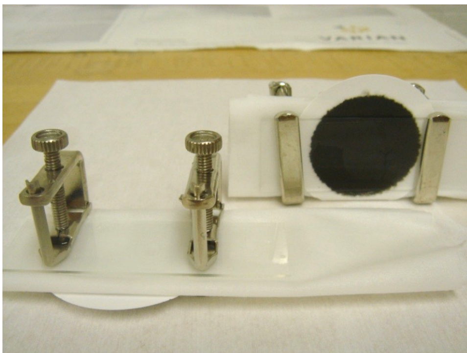
FIGURE 4.9. SWCNT films formed by the filtration method being transferred to a glass substrate. SWCNTs are filtered onto a 0.2 \mu\text{m} PTFE membrane. The film is wetted with methanol and pressed against a clean glass substrate. It is backed with a porous lint-free cloth to allow solvent wicking and evaporation.
