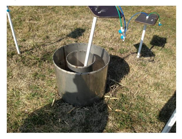
Figure 10: Double ring infiltrometer used for field attenuation study
