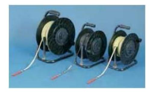
Figure 8: Water contact meters
