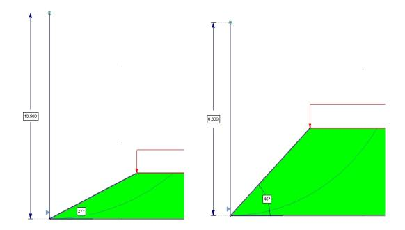
Figure 7.1: Examples of change in surface radius with change in embankment geometry (not to scale)
