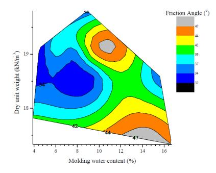
Figure 6.4: Wayne test soil friction
