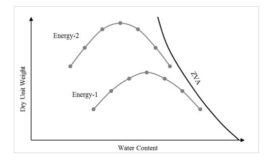
Figure 2.2: Compaction curve (adapted from Proctor, 1933)
