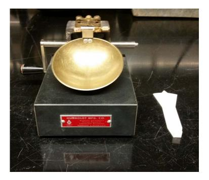
Figure 4.6: Casagrande's liquid limit cup and grooving tool
