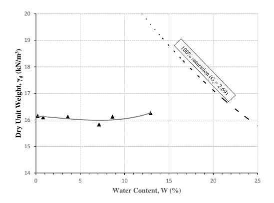
Figure 6.3: Brunswick test soil standard compaction curve
