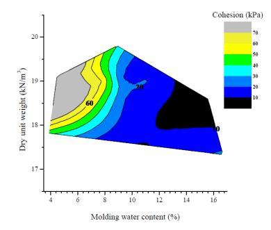
Figure 6.5: Wayne test soil cohesion
