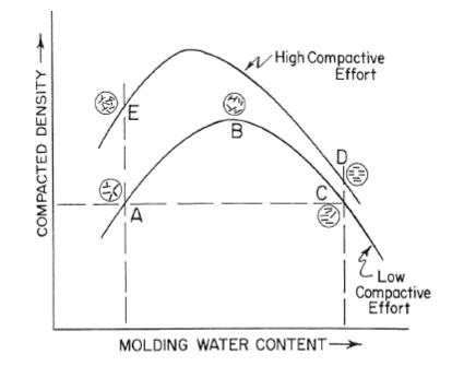
Figure 2.3: Effects of compaction on structure (adapted from Lambe, 1958)
