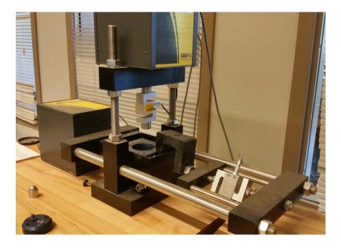
Figure 5.3: Direct shear test device
