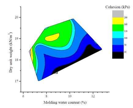
Figure 6.7: Kinston test soil cohesion
