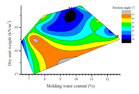
Figure 6.6: Kinston test soil friction
