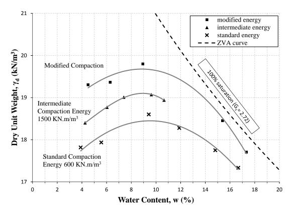
Figure 6.1: Wayne test soil compaction curves
