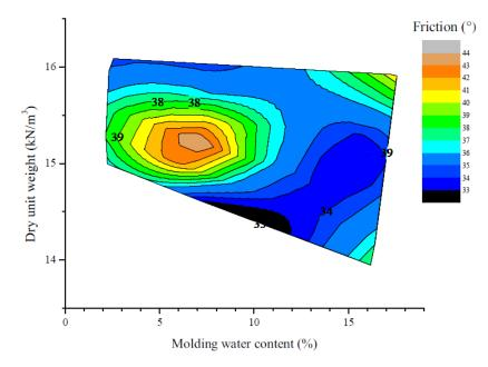
Figure 6.8: Brunswick test soil friction contours
