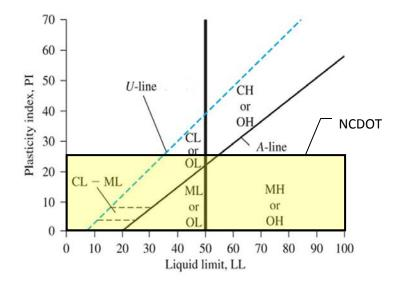
Figure 1.1: Plasticity index chart showing band of soils meeting the current NCDOT PI≤25 borrow material selection criterion
