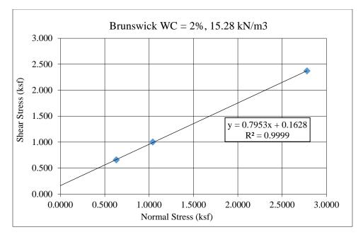
Figure 5.6: Example of shear strength envelope from a direct shear test
