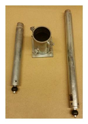
Figure 5.1: Proctor mold with standard and modified proctor hammers
