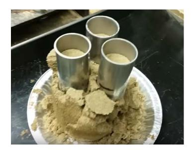
Figure 5.2: Steel tubes containing samples after removal from proctor mold
