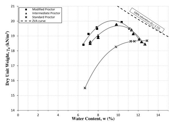
Figure 6.2 Kinston test soil compaction curves
