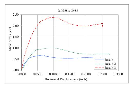
Figure 5.5: Example of shear stress versus horizontal displacement curves from three direct shear tests at three normal stress levels
