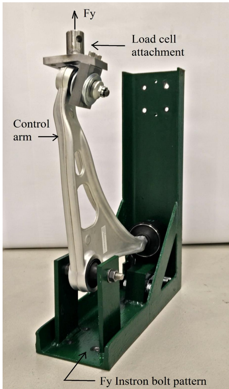
FIGURE 3.16: Setup for lateral loading
