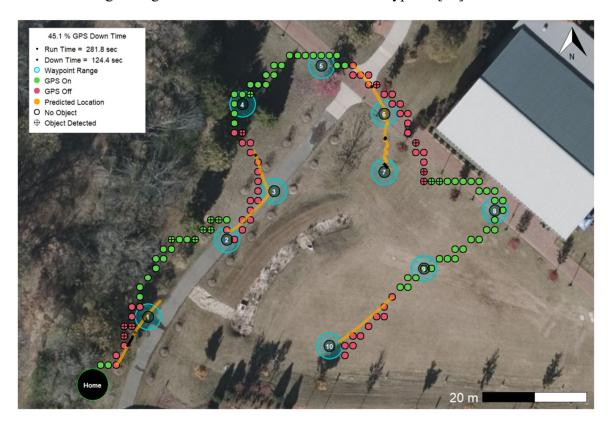
Figure 8: Autonomous Waypoint Navigation in GPS-Denied Scenario
