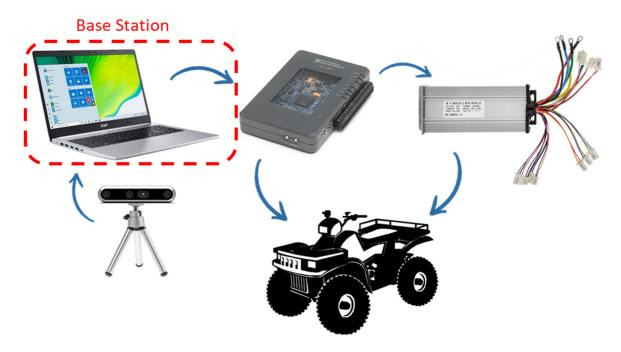
Figure 29: Hardware Configuration for Autonomous Vehicle Control
