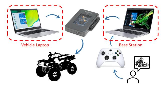
Figure 28: Hardware Configuration for Remote Vehicle Control
