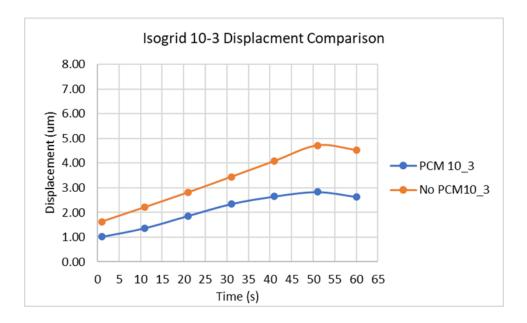
Figure 4.3.9 Variation B Maximum Deformation Comparison
