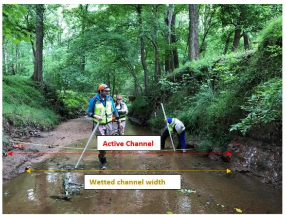
**Figure 4.5.** A transect across the channel showing the locations of the active- and wetted-channels (CMSWS 2020a).
