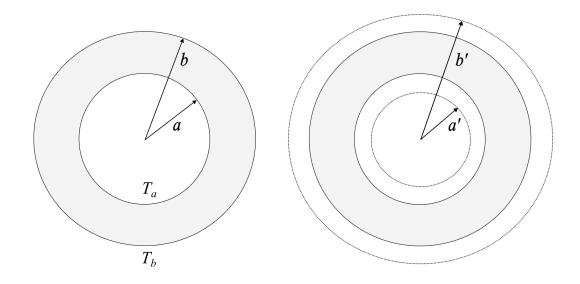
Figure 1.1: The hollow sphere before and after thermal expansion
