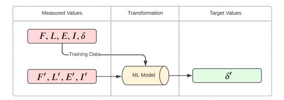
Figure 1.8: ML model training only using measurement data
