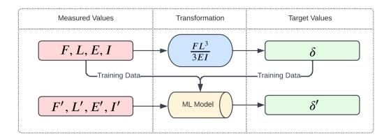
Figure 1.4: How a ML model is used to predict deflection
