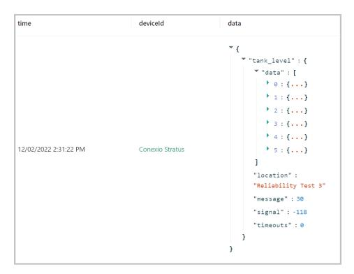
Figure 6.2: Example LightDB log entry after data transfer (Image Courtesy: Golioth IoT).
