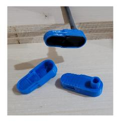
Figure 5.4: Sensor housing with potted sensor electronics.
