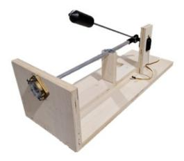
Figure 5.5: Tank level testing jig with servo positioning.
