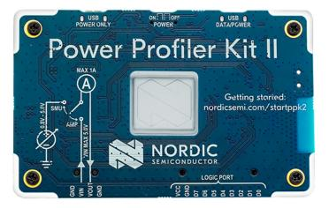
Figure 5.9: Nordic power Profiler Kit Version 2 (Image Courtesy: Nordic Semiconductor) [56].
