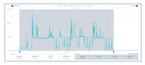
Figure 6.4: Power profile window during a cellular transmission cycle at -126 dBm.
