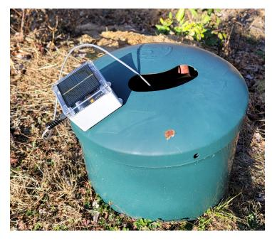
Figure 6.6: Working prototype attached with magnetic feet to an in-ground, 500 gallon tank.
