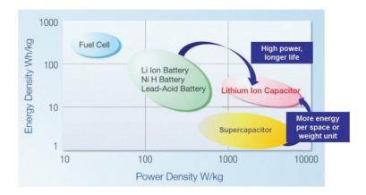
Figure 5.7: Ragonne plot of different energy storage technologies, including LIC characteristics compared to LIB and EDLC [55].
