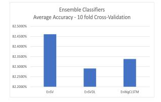
Figure 5.3: Ensemble classifier accuracy graph. EnSV had a higher accuracy than either EnWgCLSTM or EnSVDL, indictating inclusion of traditional machine learning algorithms may add value.
