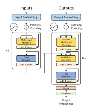
Figure 2.2: Architecture of a Transformer neural network [74].
