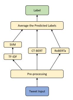
Figure 2.5: Ensemble architecture model used by Babu and Eswari for binary text classification.
