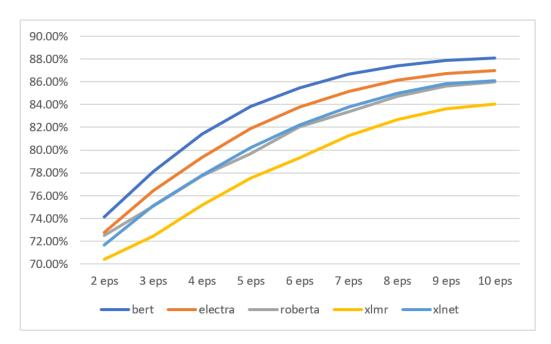
Figure 8.1: TL accuracy increase curve flattens at 8-10 fine-tuning epochs.
