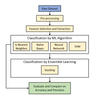
Figure 2.6: Ensemble architecture assessed by Lai, Chan, and Chin for sarcasm detection.
