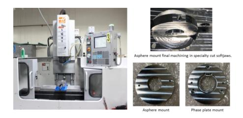
Figure 4-4: A HAAS CNC Toolroom Mill with manufactured mountings.
