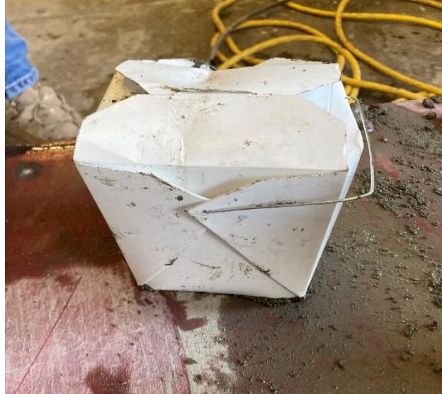
Figure 3.7: Takeout container after being filled with concrete
