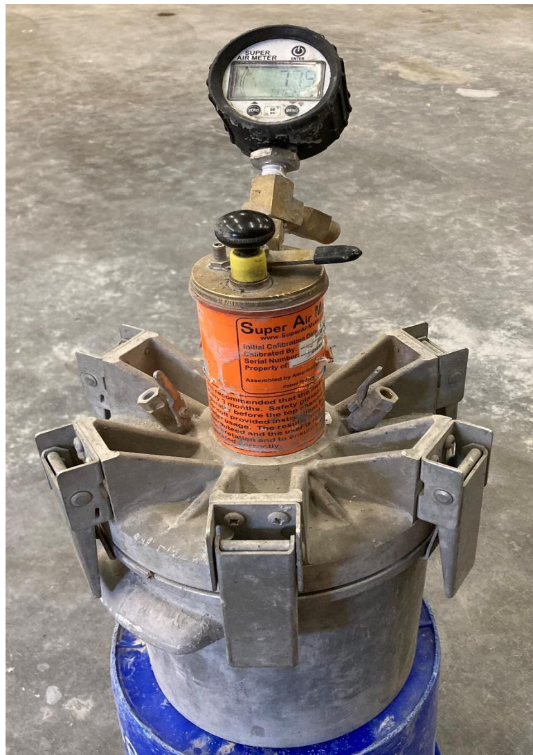
Figure 3.5: Super Air Meter (SAM)
