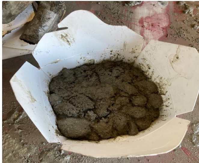
Figure 3.6: Sample being cast in takeout container
