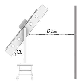
Figure 12: Tilted solar simulator diagram
