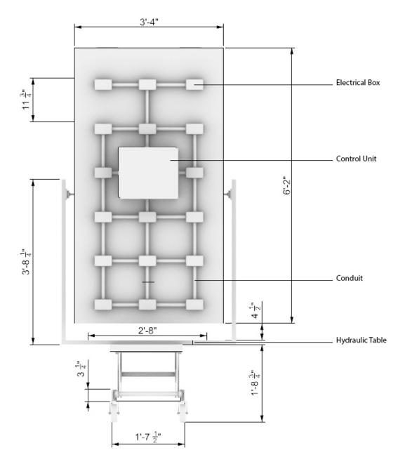
Figure 6: Solar Simulator Component
