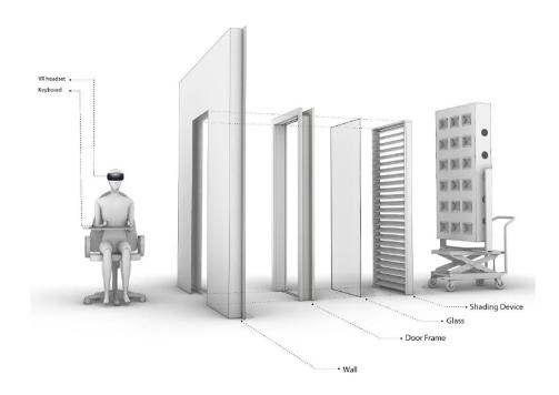
Figure 18: Testbed Components
