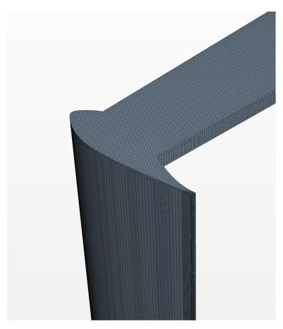
Figure 4.22: Isometric view of surface mesh on turbine blades
