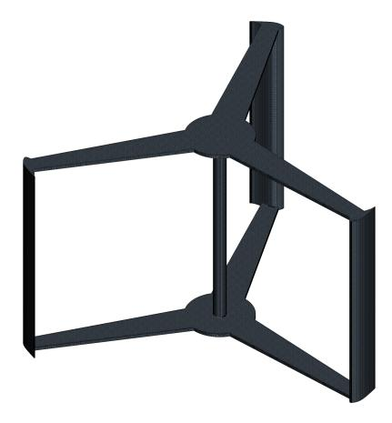
Figure 4.20: Isometric view of surface mesh over single turbine system
