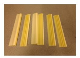
Figure 4.7: 3D printed turbine blades
