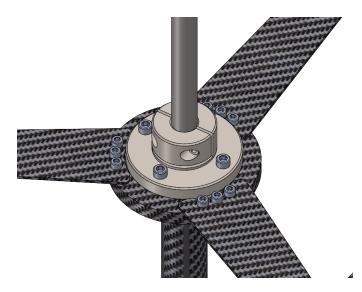
Figure 4.9: Central hub for turbine rotor
