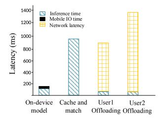
Figure 5.17: The end-to-end delay of classification application.
