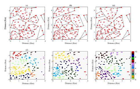
Figure 6.8: The visualization of network partitioning. (9 (a), (b) and (c): BS-based network partition at 8:00, 14:00 and 20:00, respectively; 9 (d), (e) and (f): grid-based network partition at 8:00, 14:00 and 20:00, respectively.) high layer in the clustering tree without clustering the whole network again. Thus,
