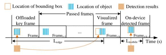
Figure 5.6: The pipeline of a real MAR system.
