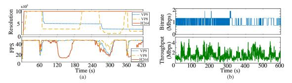
Figure 3.2: The performance of the WebRTC system (a) and ABR based live video streaming system (b).
