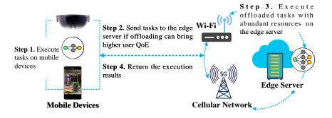
Figure 1.5: The system of edge-based MAR applications.
