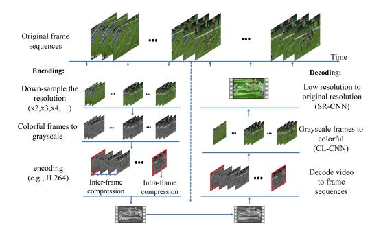
Figure 4.5: The video encoding scheme.
