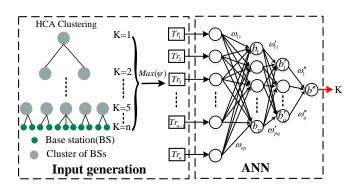
Figure 6.9: The structure of the neural network predictor.
