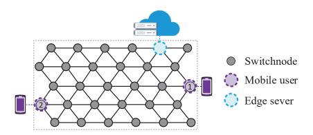
Figure 5.16: The network topology of the simulated network. 5.6.3.2 Experiment Results Analysis
