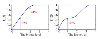
Figure 3.3: CDF of bitrate level and frame latency.
