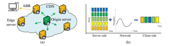
Figure 1.1: The content distributed network system (a) and the adaptive bitrate selection algorithm (b).
