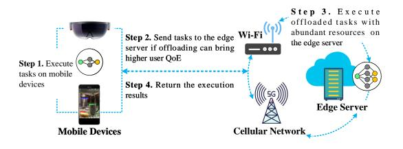
Figure 5.2: The system of edge-based MAR applications.
