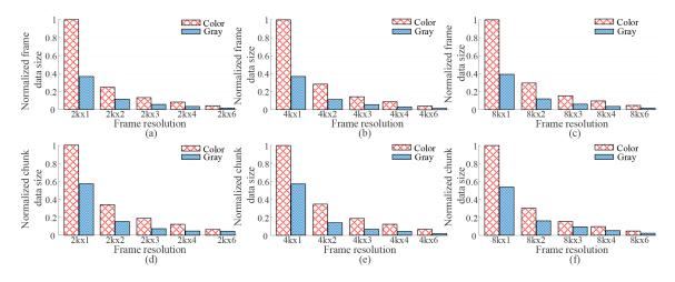
Figure 4.8: The normalized video frame and chunk data size.
