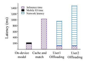
Figure 5.18: The end-to-end delay of object detection application. the edge server. The reason is that the cache size is limited, not all the objects will be successfully matched.
