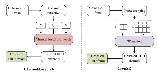
Figure 4.7: The framework of super resolution models.
