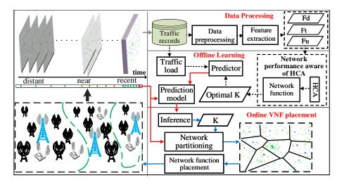
Figure 6.2: The data-driven virtual network function placement framework. 6.1.1 Data Processing
