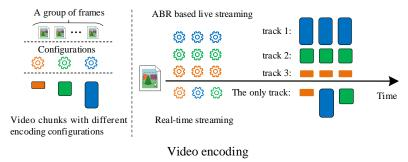
Figure 3.1: The live video streaming system.
