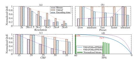
Figure 3.4: The impact of video encoding parameters on QoE metrics.
