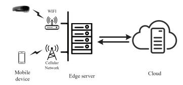
Figure 1.3: The cloud/edge-based mobile AR system.
