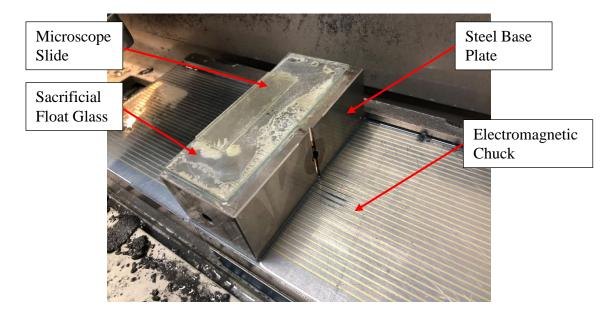
Figure 89. Steel block, float glass, and microscope slide waxed down on magnetic chuck, ready for creep feed grinding.
