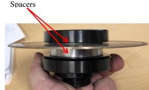
Figure 87. Front view of metal bonded diamond wheel mounted in arbor.
