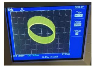
Figure 53. Lissajous figure of the MOD arm mirror over a five minute measurement time
