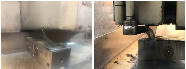
*Figure 90. Flood coolant during operation, front view.*
