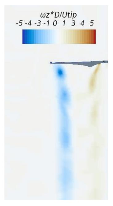
Figure 20: Mean vorticity of 7200 RPM case.
