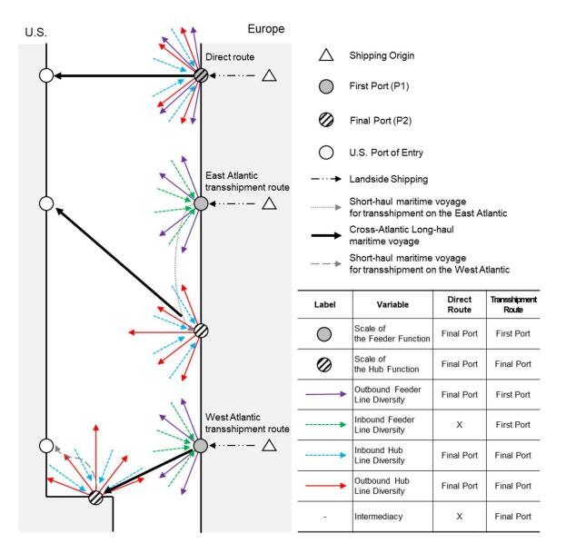
Figure 2-3 Hub-and-spoke configuration variables measured on forwarding and final ports
