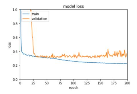
Figure 5.14: Diagnostic plot of Vanilla LSTM RNN showing an overfitting model
