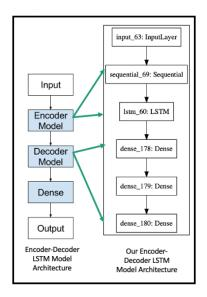
Figure 5.13: Vanilla Encoder-Decoder LSTM Network
