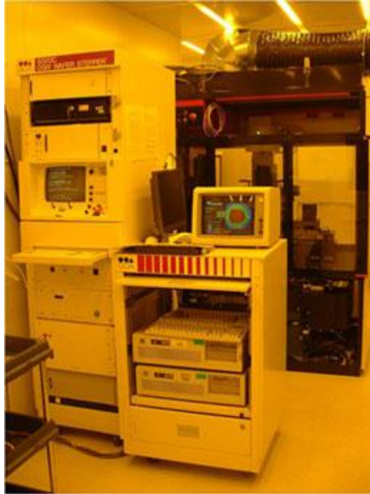
Figure 11:2 GCA6300-C G-line (436nm) stepper control unit and the stepper system.
