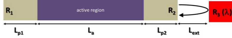
Figure 1:5 Schematic illustration of external cavity with a external dispersive feedback element. The reflectivity of the filter is peaked at a specific wavelength.
