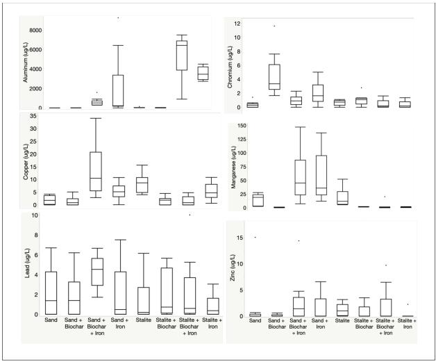
Figure 6. Phase 4.1 spiked stormwater effluent - aluminum, copper, manganese, chromium, lead and zinc.
