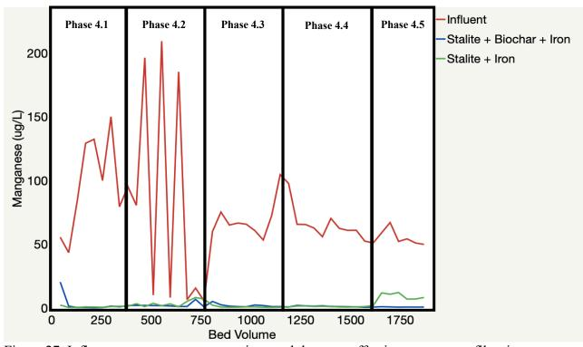
Figure 27. Influent manganese concentrations and the most effective stormwater filtration system effluent (Stalite + iron and Stalite + biochar + iron) through all phases. Phases are outlined by bed volumes experienced in each phase (outline is approximate).
