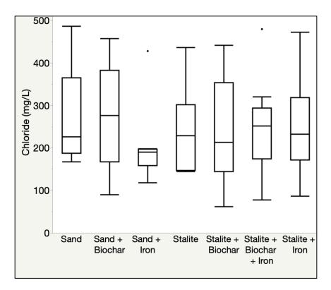
Figure 17. Phase 4.4 spiked stormwater effluent – Chloride.
