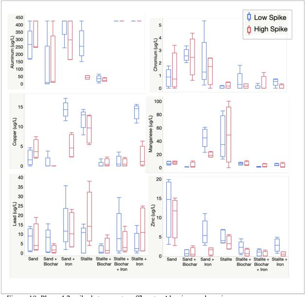
Figure 10. Phase 4.2 spiked stormwater effluent – Aluminum, chromium, copper, manganese, lead and zinc.
