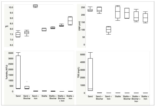
Figure 19. Phase 4.5 spiked stormwater effluent – pH, ORP, turbidity and TSS.
