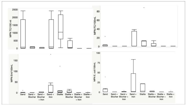
Figure A1. Phase 4.1 spiked stormwater effluent – Total coliform, fecal coliform, E. coli, and enterococci.
