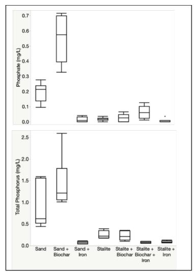
Figure 20. Phase 4.5 spiked stormwater effluent – Total phosphorus and phosphate as P.
