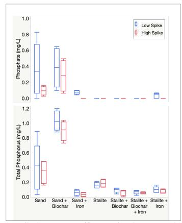
Figure 8. Phase 4.2 spiked stormwater effluent – Phosphate as P and total phosphorus.
