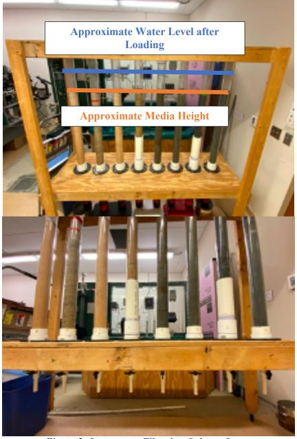
Figure 2. Stormwater Filtration Column Setup
