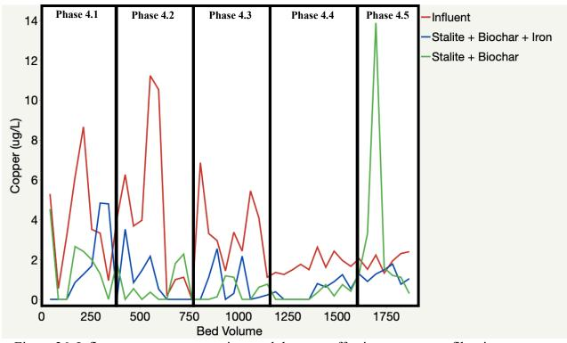
Figure 26. Influent copper concentrations and the most effective stormwater filtration system effluent (Stalite + biochar and Stalite + biochar + iron) through all phases. Phases are outlined by bed volumes experienced in each phase (outline is approximate).
