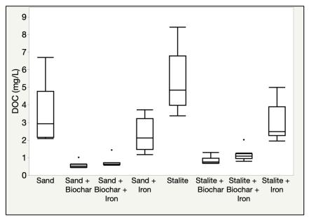
Figure A3. Phase 4.1 spiked stormwater effluent - Dissolved organic carbon.
