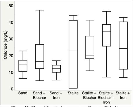
Figure 13. Phase 4.3 spiked stormwater effluent – Chloride.
