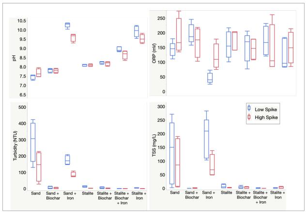
Figure 7. Phase 4.2 spiked stormwater effluent – pH, ORP, turbidity, and TSS.
