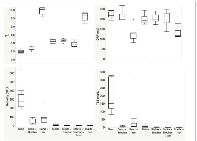
Figure 11. Phase 4.3 spiked stormwater effluent – pH, ORP, turbidity and TSS.
