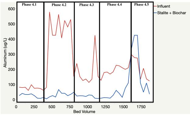
Figure 24. Influent aluminum concentrations and the most effective stormwater filtration system effluent (Stalite + biochar) through all phases. Phases are outlined by bed volumes experienced in each phase (outline is approximate).
