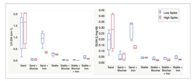
Figure A4. Phase 4.2 spiked stormwater effluent – UV-254 and SUVA.
