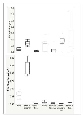
Figure 12. Phase 4.3 spiked stormwater effluent – Total phosphorus and phosphate as P.
