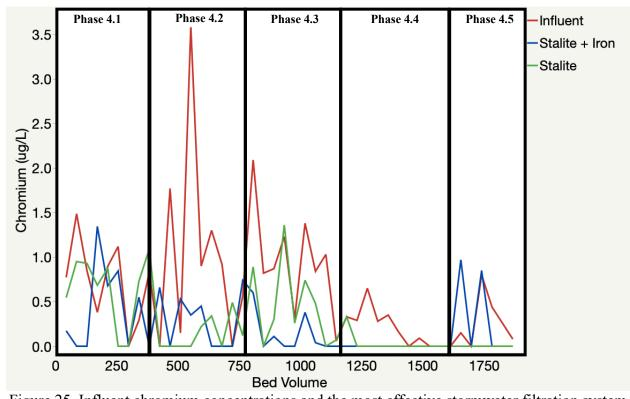
Figure 25. Influent chromium concentrations and the most effective stormwater filtration system effluent (Stalite + iron and Stalite) through all phases. Phases are outlined by bed volumes experienced in each phase (outline is approximate).
