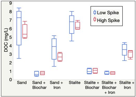
Figure A5. Phase 4.2 spiked stormwater effluent – DOC.
