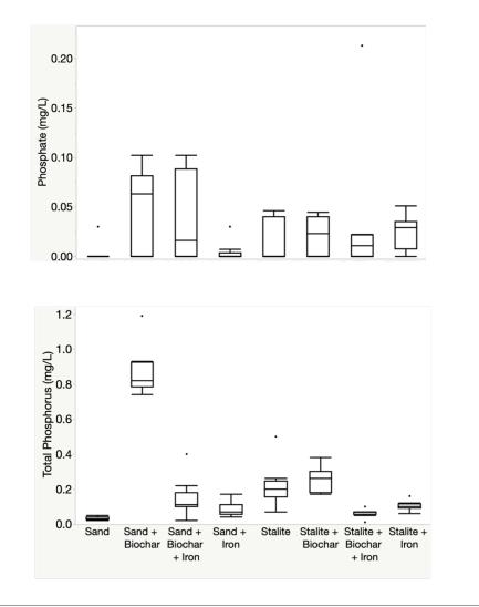
Figure 4. Phase 4.1 spiked stormwater effluent - Total phosphorus and phosphate as P.
