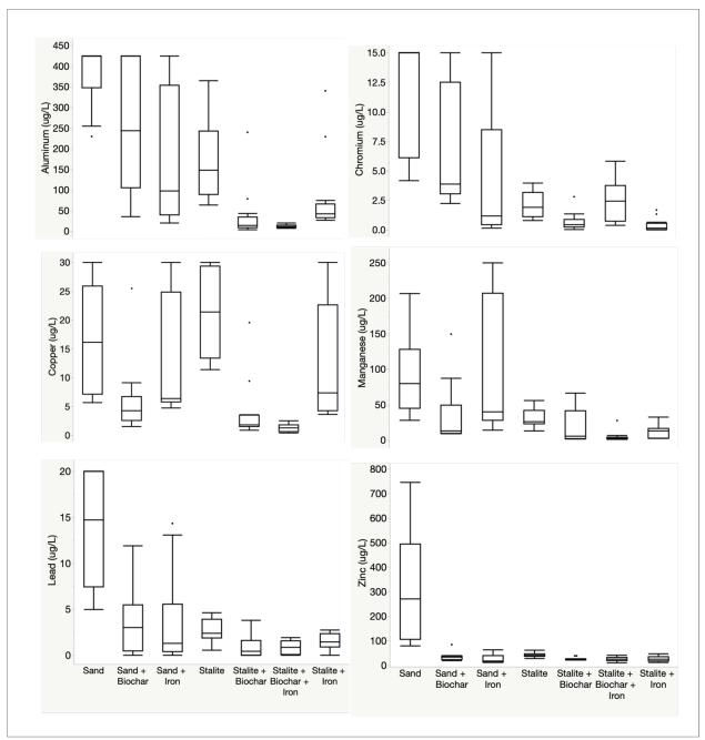
Figure 23. Total recoverable metals effluent - Total aluminum, chromium, copper, manganese,
