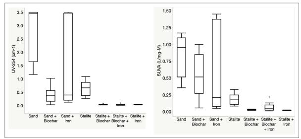
Figure A10. Phase 4.4 spiked stormwater effluent – UV-254 and SUVA.
