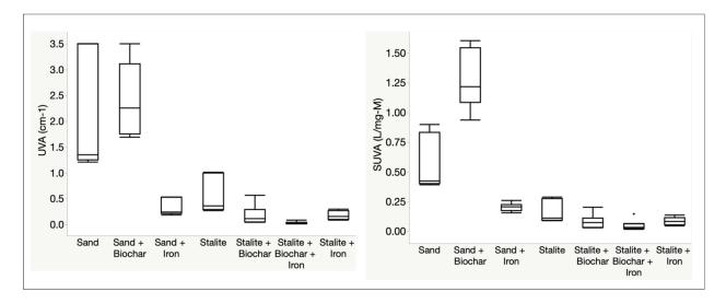
Figure A13. Phase 4.5 spiked stormwater effluent – UV-254 and SUVA.
