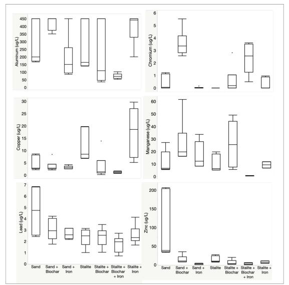
Figure 22. Phase 4.5 spiked stormwater effluent – Aluminum, chromium, copper, manganese,
