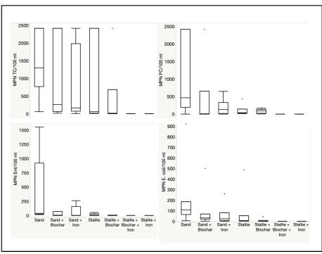
Figure A6. Phase 4.3 spiked stormwater effluent - Total coliform, fecal coliform, E. coli, and
