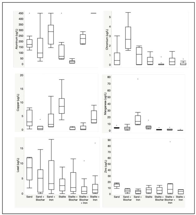
Figure 14. Phase 4.3 spiked stormwater effluent – Aluminum, chromium, copper, manganese,
