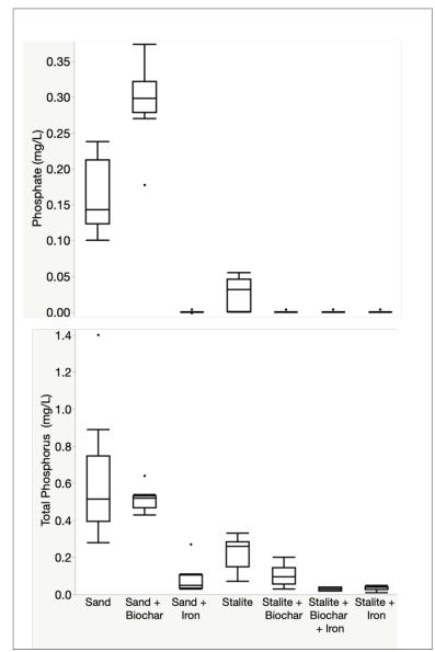
Figure 16. Phase 4.4 spiked stormwater effluent – Total phosphorus and phosphate as P.
