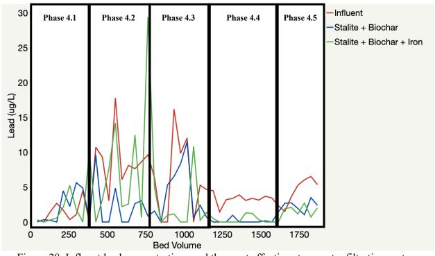
Figure 28. Influent lead concentrations and the most effective stormwater filtration system effluent (Stalite + biochar and Stalite + biochar + iron) through all phases. Phases are outlined by bed volumes experienced in each phase (outline is approximate).
