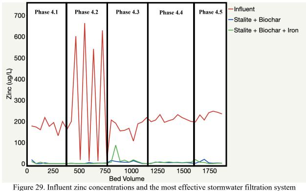
effluent (Stalite + biochar and Stalite + biochar + iron) through all phases. Phases are outlined by bed volumes experienced in each phase (outline is approximate).
