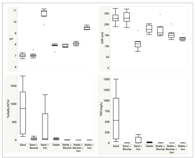
Figure 15. Phase 4.4 spiked stormwater effluent – pH, ORP, turbidity and TSS.
