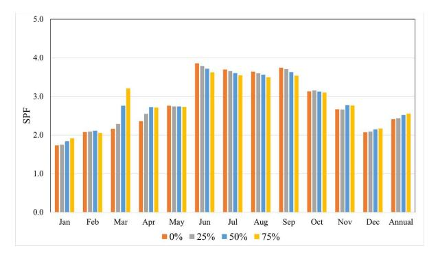
Figure 6-9: Comparison of the SPF for systems with different percentages of the tank volume used by the PCM module having a melting temperature of 10°C (Baltimore)
