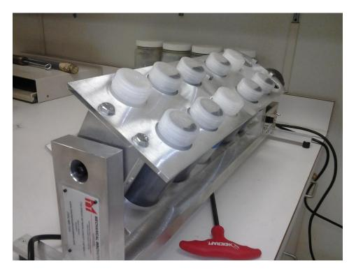
FIGURE 6-1: pH dependence test experimental setup
