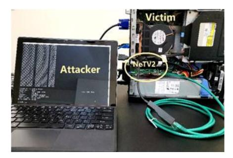
Figure 3.1: Setup for the PCIleech attack.
