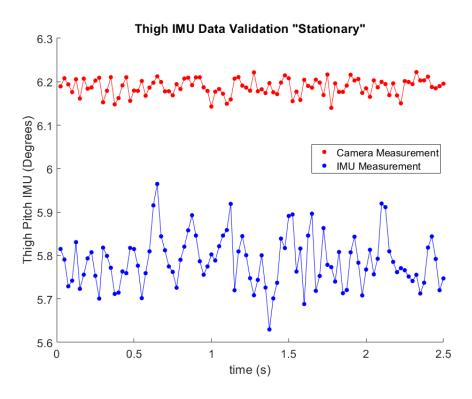
Figure 5.17: Test 2 of stationary position of thigh IMU.
