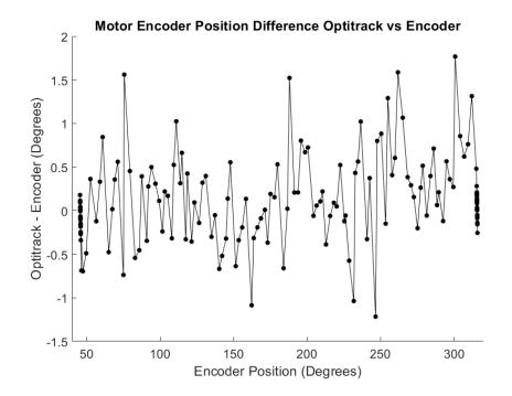
Figure D.5: Trial 5: Motor in-motion difference in measured angle.
