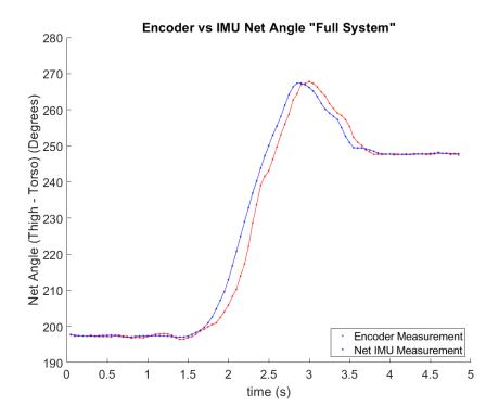
Figure E.1: Trial 1: Full system operation - IMU vs. encoder position.
