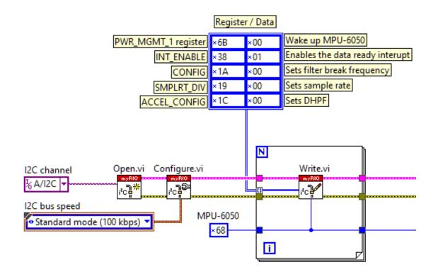
A.2 Reading MPU-6050 raw data over I2C
