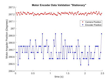
Figure 5.10: Motor stationary data from dataset 23.
