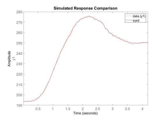
Figure 5.35: Loaded System state-space model comparison.
