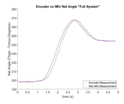
Figure E.9: Trial 9: Full system operation - IMU vs. encoder position.
