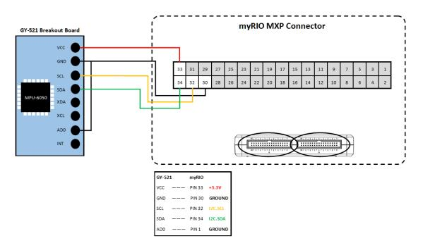
Figure 4.1: IMU to myRIO MXP wiring diagram.
