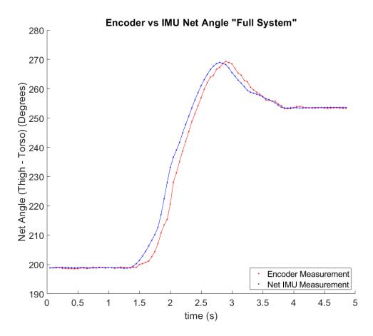
Figure 5.22: Trial 2: Full system operation - IMU vs. encoder position.
