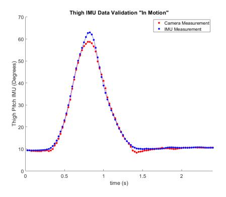
Figure 5.11: In-motion data of thigh position from dataset 1.
