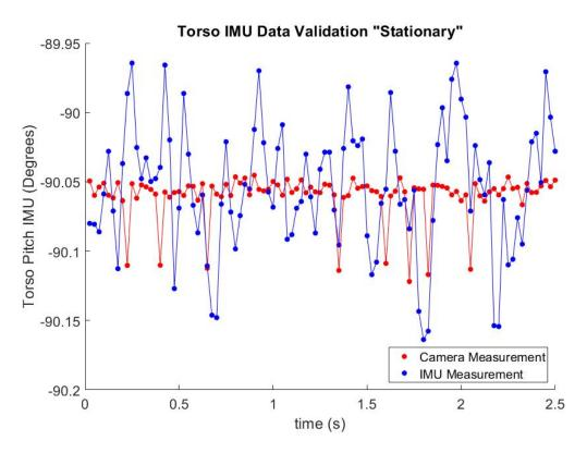
Figure 5.16: Test 1 of stationary position of torso IMU.
