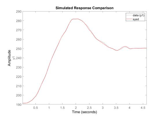
Figure 5.26: No-load state-space model compared to no-load system.
