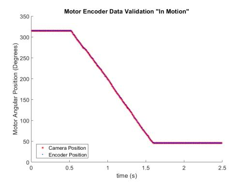
Figure 5.5: Motor position when rotating from 315 to 45 degrees.
