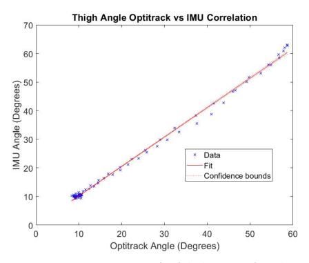
Figure 5.13: In-motion regression fit of thigh position from dataset 1.
