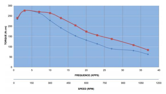
Figure 3.6: 24HS39-4204D pull out torque specification chart.
