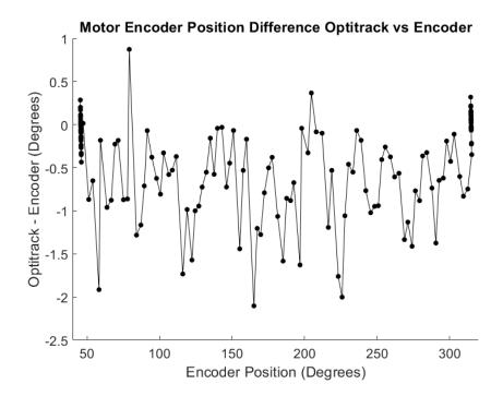
Figure D.10: Trial 10: Motor in-motion difference in measured angle.
