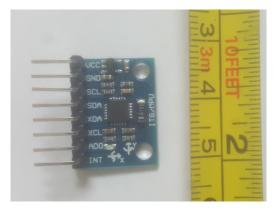
Figure 3.2: GY-521 breakout board containing MPU-6050 IMU.
