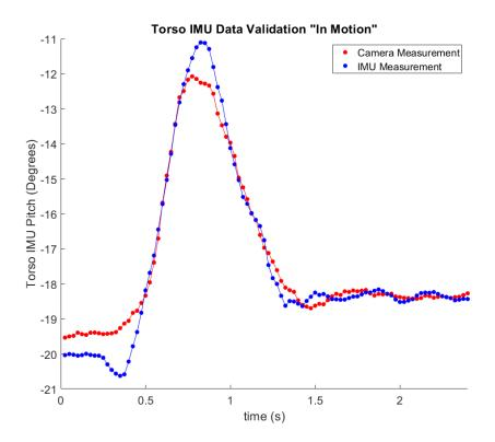
Figure 5.12: In-motion data of torso position from dataset 1.
