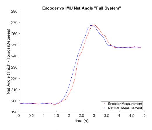
Figure 5.19: Trial 1: Full system operation - IMU vs. encoder position.
