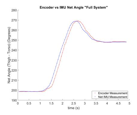
Figure E.5: Trial 5: Full system operation - IMU vs. encoder position.
