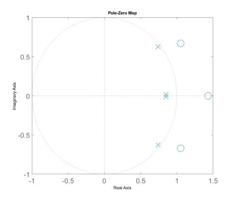
Figure 5.36: Loaded System pole-zero plot of discrete model, T(z).
