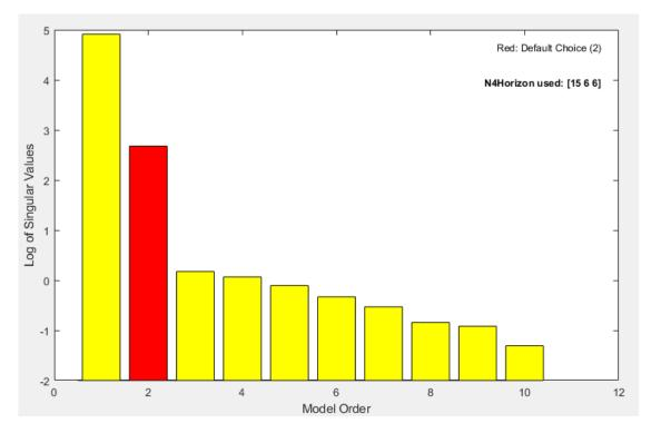
Figure 5.25: MATLAB results used to determine optimal system order.
