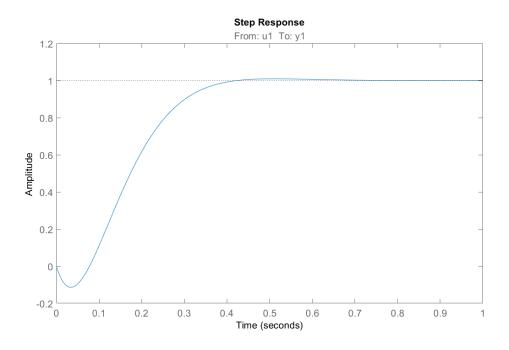
Figure 5.32: No-load step response of T(s).
