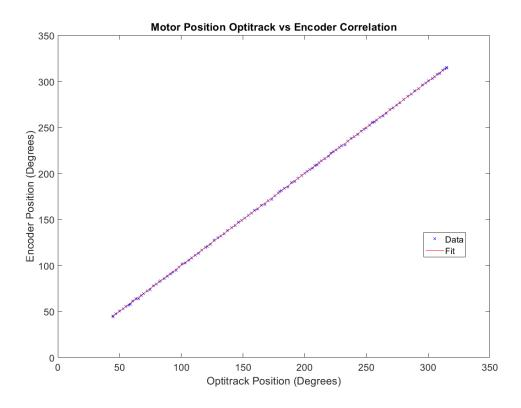
Figure 5.7: Regression curve of motor position measurements.
