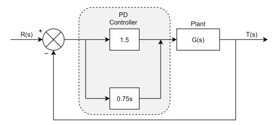
Figure 5.29: Initial block diagram of the control system
