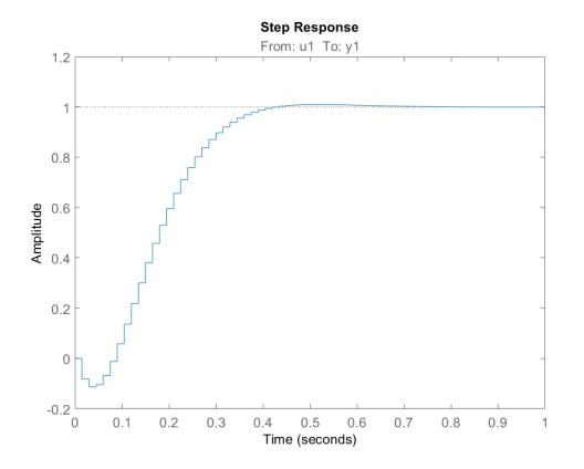
Figure 5.28: No-load state-space model step response.
