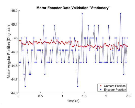
Figure 5.8: Stationary position of motor seen by encoder and cameras.
