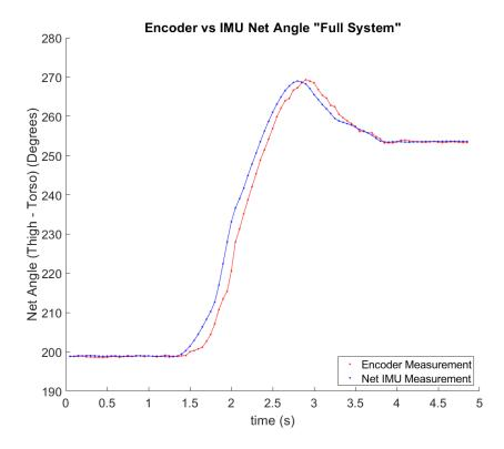
Figure E.2: Trial 2: Full system operation - IMU vs. encoder position.
