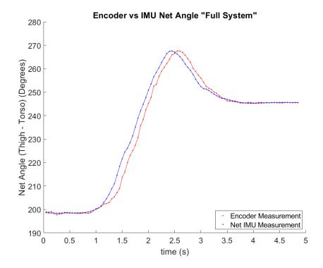
Figure E.8: Trial 8: Full system operation - IMU vs. encoder position.
