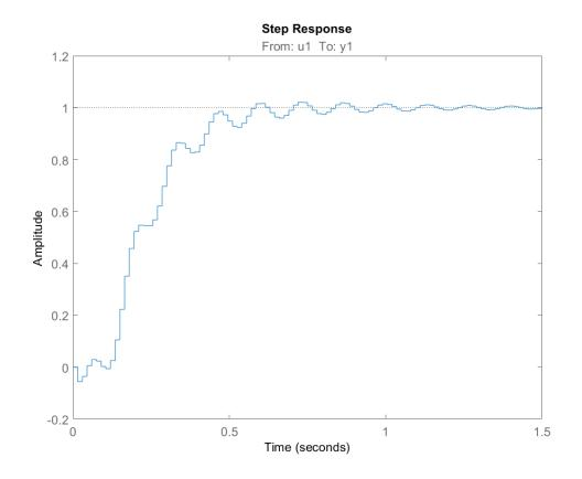
Figure 5.37: Loaded system step response of discrete model, T(z)'.
