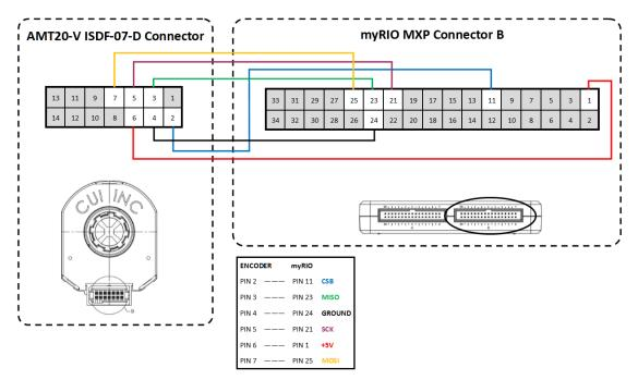
Figure 4.5: AMT20-V encoder to myRIO wiring diagram.
