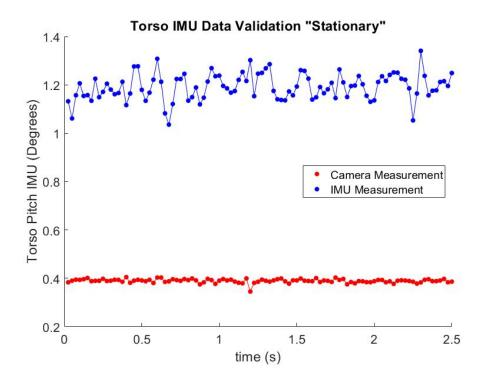
Figure 5.18: Test 2 of stationary position of torso IMU.
