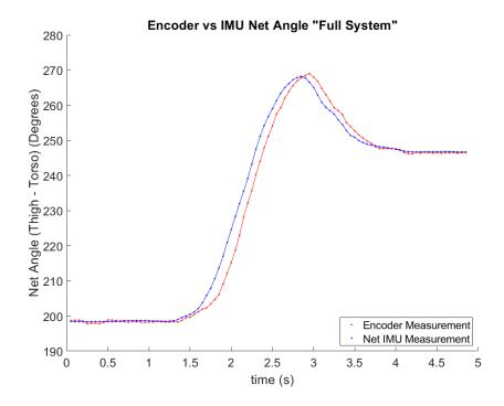
Figure E.6: Trial 6: Full system operation - IMU vs. encoder position.
