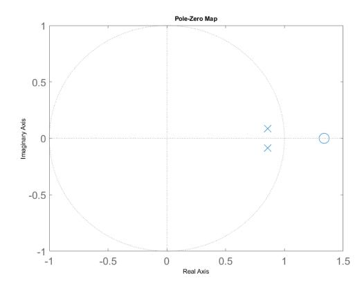
Figure 5.27: No-load pole-zero plot of discrete-time system, T(z).
