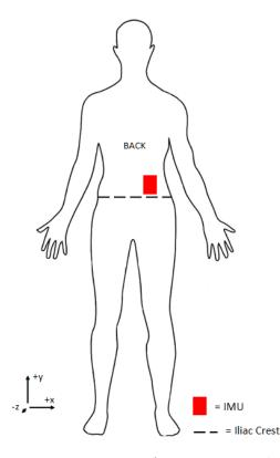
Figure 3.4: Location of torso mounted IMU.
