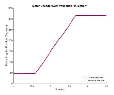
Figure 5.4: Motor position when rotating from 45 to 315 degrees.
