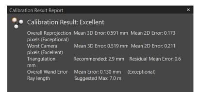
Figure 5.1: Motive calibration results for encoder data validation.
