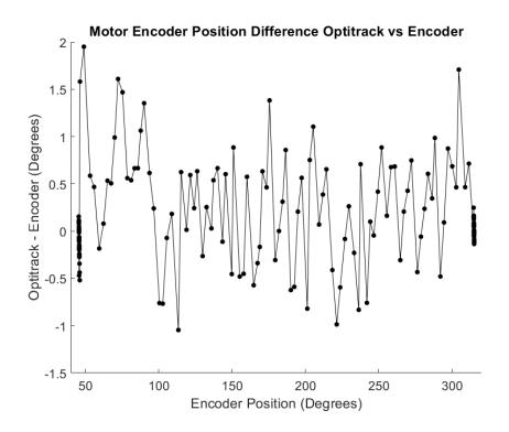
Figure D.3: Trial 3: Motor in-motion difference in measured angle.
