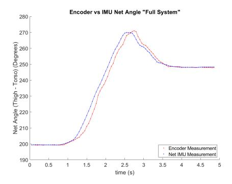
Figure E.4: Trial 4: Full system operation - IMU vs. encoder position.
