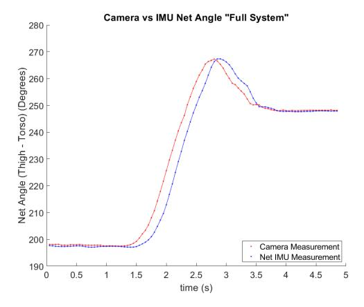
Figure 5.21: Trial 1: Full system operation - IMU vs. camera position.
