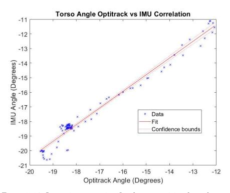
Figure 5.14: In-motion regression fit of torso position from dataset 1.
