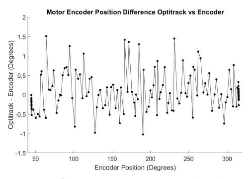
Figure 5.6: Difference in motor position between encoder and cameras.
