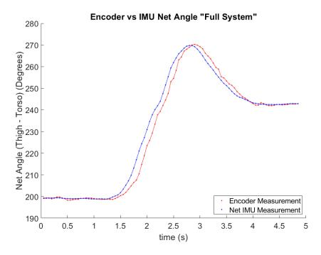
Figure E.7: Trial 7: Full system operation - IMU vs. encoder position.
