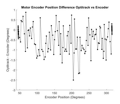
Figure D.8: Trial 8: Motor in-motion difference in measured angle.
