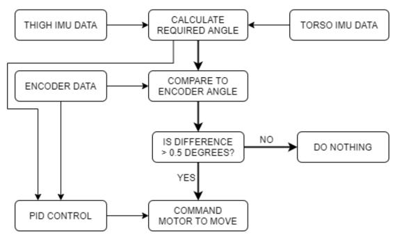
Figure 4.6: Flow of data for motor control and decision making.
