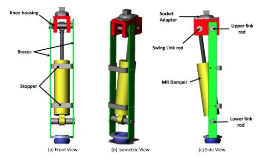
Figure 2.4: Electronic below-knee prosthesis [4]
