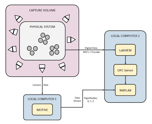
Figure 4.10: Data validation flow into MATLAB.
