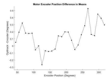
Figure 5.9: Difference in means of all stationary motor datasets
