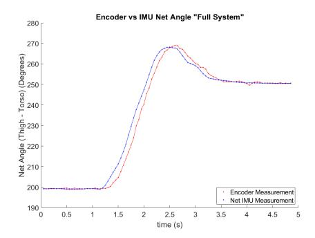
Figure E.3: Trial 3: Full system operation - IMU vs. encoder position.
