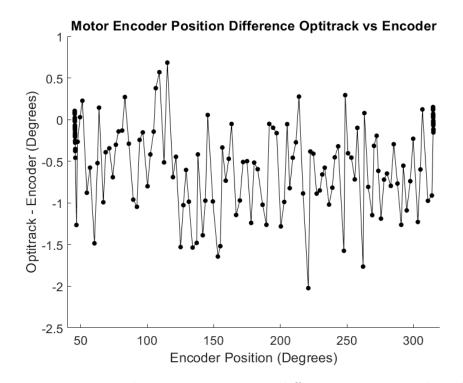
Figure D.2: Trial 2: Motor in-motion difference in measured angle.
