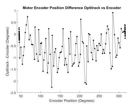
Figure D.6: Trial 6: Motor in-motion difference in measured angle.
