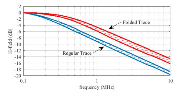
Figure 1.4: Normalized magnetic field distribution with respect to frequency for the simulations results in Figure 1.3 for different positions of the sensor element on the current carrying trace in regular and folded trace configuration.
