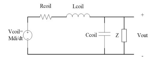
Figure 3.6: Equivalent circuit diagram of a Rogowski coil
