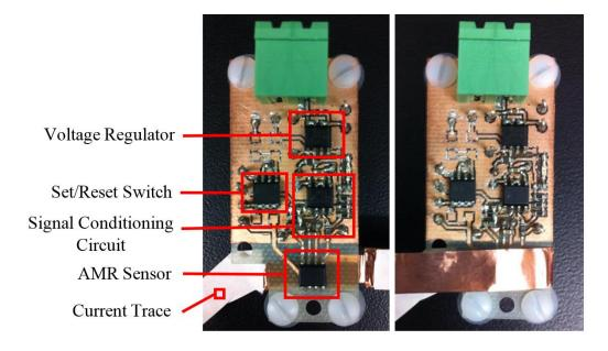
Figure 1.6: Hardware setup for evaluation of the AMR current sensor. Left: standard scheme, Right: sensing scheme with the folded trace technique.
