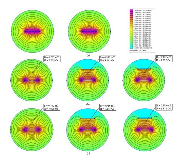
Figure 2.2: Simulation results for the effect of MCON on magnetic field distribution for 10A current at (a) DC, (b) 5MHz with No MCON (left), 1mil Cu MCON (middle) and 5mil Cu MCON (right), (c) 5MHz with No MCON (left), 5mil Al MCON (middle) and 10mil Al MCON (right)
