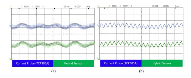
Figure 3.15: Performance of the proposed wideband AMR-Rogowski current sensor in measuring high frequency inverter output current compared to a current probe: (a) regular and (b) zoomed
