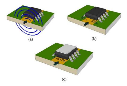
Figure 2.1: The concept visualization: (a) Magnetic field distribution at low frequencies,(b) Magnetic field distribution at high frequencies due to skin effect, (c) Magnetic field distribution with the proposed magnetic concentrator (MCON)
