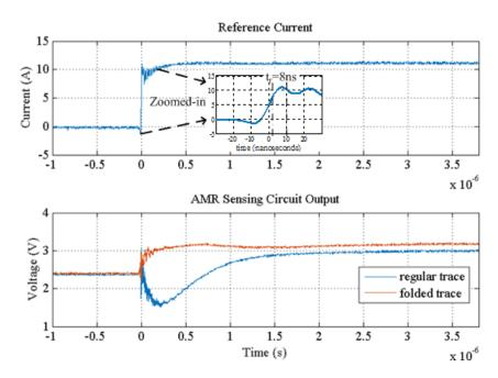
Figure 1.7: Experimental Results: step response comparison of the AMR sensing circuit for regular trace and the proposed folded trace implementation.
