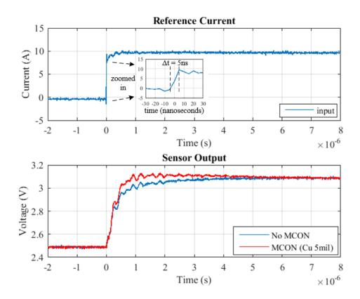
Figure 2.9: Comparison of AMR sensor response for 10A step current with no MCON and 5 mil copper MCON
