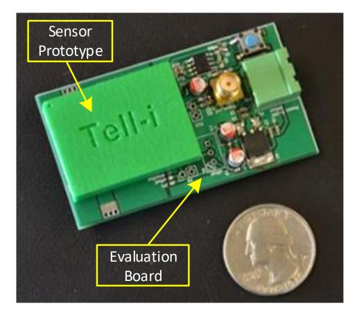
Figure 3.7: Developed hardware prototype of the proposed wideband current sensor with custom designed evaluation board.
