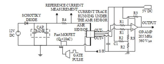
Figure 1.5: Circuit diagram of the set-up for testing the AMR sensing scheme.
