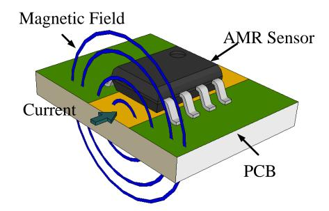
Figure 1.1: General layout, i.e. "standard configuration" of AMR sensor for current measurement.
