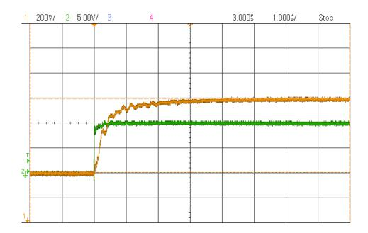
Figure 2.7: Response of the AMR sensor with respect to 10A step current with no MCON. Scales - X-axis: 1us/div, Y-axis: 5v/div (green), 200mv/div (yellow)
