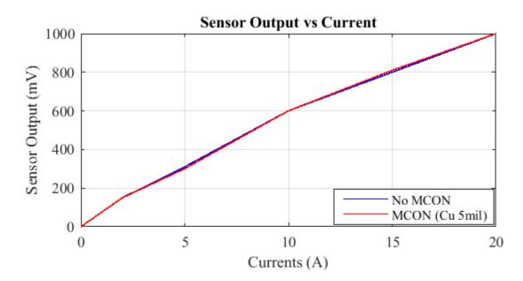
Figure 2.13: Change (offset 2.5V) in steady state sensor output with step currents of different magnitude for no MCON and 5 mil copper MCON
