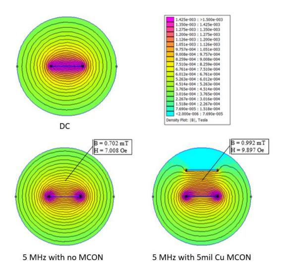
Figure 3.5: Simulation results for 5mil copper MCON on magnetic field distribution at 10A current
