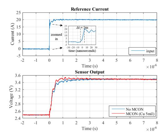
Figure 2.12: Comparison of AMR sensor response for 20A step current with no MCON and 5 mil copper MCON
