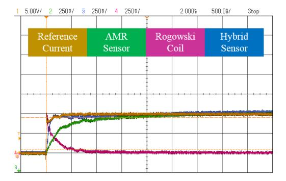
Figure 3.11: Hybrid sensor response for a fast 10A step current.
