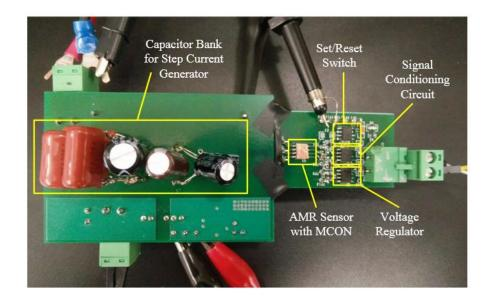
Figure 2.6: Experimental setup with step current generator and AMR sensor equipped with 1 mil copper MCON
