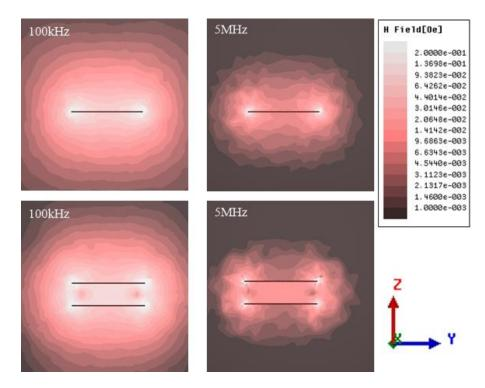
Figure 1.3: Simulation results: magnetic field distribution of bare trace (top) and folded trace (bottom) at two different frequencies.
