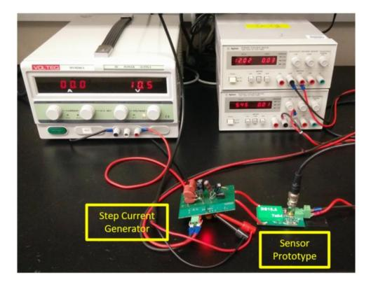
Figure 3.9: Test circuits and experimental setup used for the step current test
