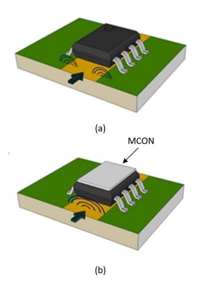
Figure 3.4: Planar Magnetic Concentrator (MCON) concept: (a) Magnetic field distribution at high frequencies due to skin effect and (b) Magnetic field distribution with MCON
