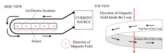
Figure 1.2: Proposed folded trace technique to normalize and intensify the field.
