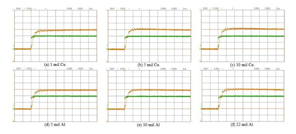
Figure 2.8: Improvement in the response of the AMR sensor with respect to 10A step current with 6 different MCONs. Scales - X-axis: 1us/div, Y-axis: 5v/div (green), 200mv/div (yellow)
