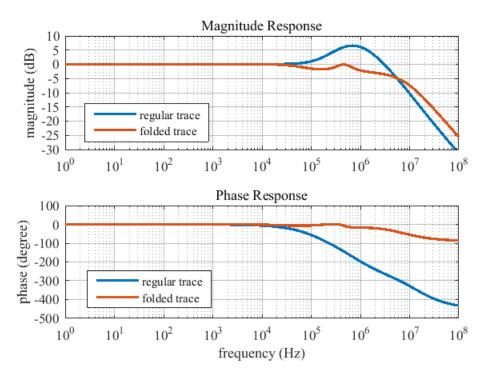
Figure 1.8: Frequency Analysis (normalized) of AMR sensor with Regular (Bare) Trace and Folded Trace based on the experimental results shown in Figure 1.7.
