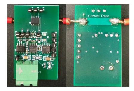
Figure 2.5: Prototype board for AMR sensor evaluation with the sensor and the current trace on opposite sides of the PCB
