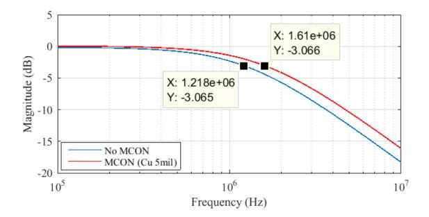
Figure 2.15: Frequency response showing the bandwidth improvement for the step current response presented in Figure 2.12 for no MCON and 5 mil copper MCON
