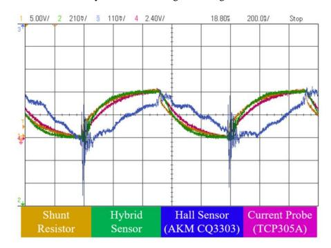
Figure 3.14: Different sensor responses for inductor current measurement in a 1MHz half bridge converter.
