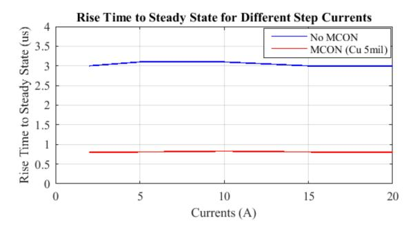
Figure 2.14: Change in rise time to steady state for sensor output with step current of different magnitudes for no MCON and 5 mil copper MCON
