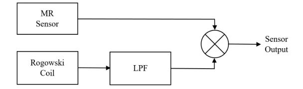
Figure 3.3: Simplified block diagram of the proposed wideband Magnetoresistor-Rogowski hybrid current sensing scheme.
