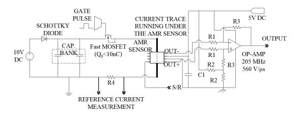
Figure 2.4: Circuit diagram of the hardware setup for evaluation of the performance of the AMR sensor equipped with different MCONs.
