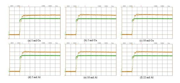
Figure 2.11: Improvement in the response of the AMR sensor with respect to 20A step current with 6 different MCONs. Scales - X-axis: 1us/div, Y-axis: 5v/div (green), 200mv/div (yellow)
