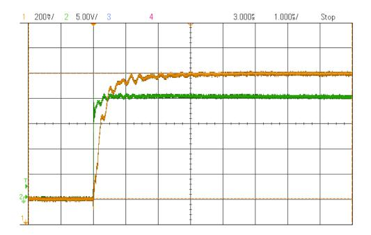
Figure 2.10: Response of the AMR sensor with respect to 20A step current with no MCON. Scales - X-axis: 1us/div, Y-axis: 5v/div (green), 200mv/div (yellow)
