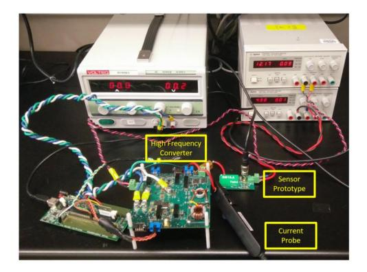
Figure 3.10: Test circuits and experimental setup used for the converter test
