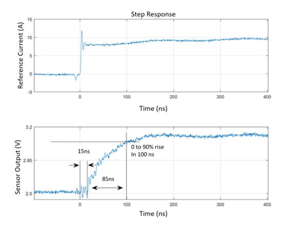
Figure 3.12: Hybrid sensor response for 10A step current (zoomed).
