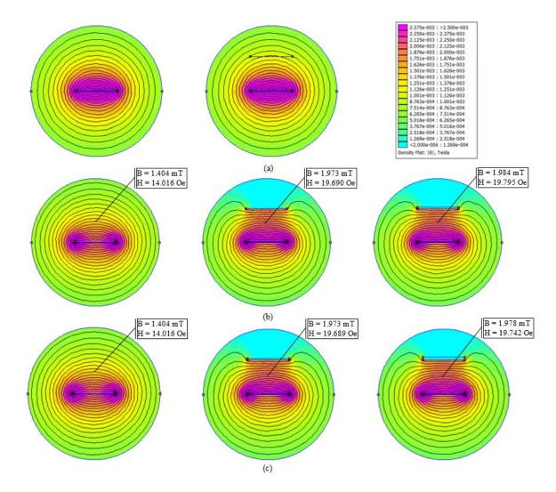
Figure 2.3: Simulation results for the effect of MCON on magnetic field distribution for 20A current at (a) DC, (b) 5MHz with No MCON (left), 1mil Cu MCON (middle) and 5mil Cu MCON (right), (c) 5MHz with No MCON (left), 5mil Al MCON (middle) and 10mil Al MCON (right)
