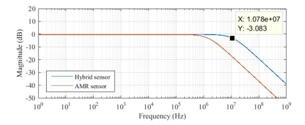
Figure 3.13: Frequency response for the step current response shown in Figure 3.11.
