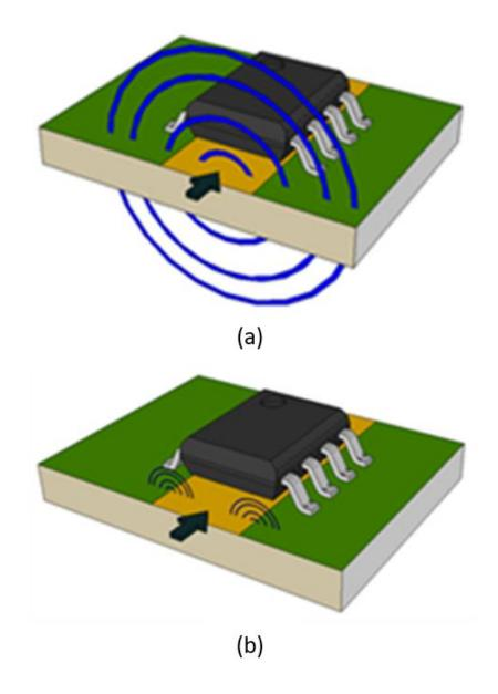
Figure 3.1: Magnetic field distribution generated by current in a PCB trace at: (a) low frequencies and (b) high frequencies
