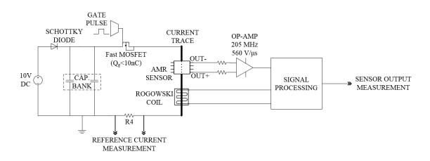
Figure 3.8: Test circuit diagram of the proposed wideband AMR-Rogowski hybrid current sensing scheme.
