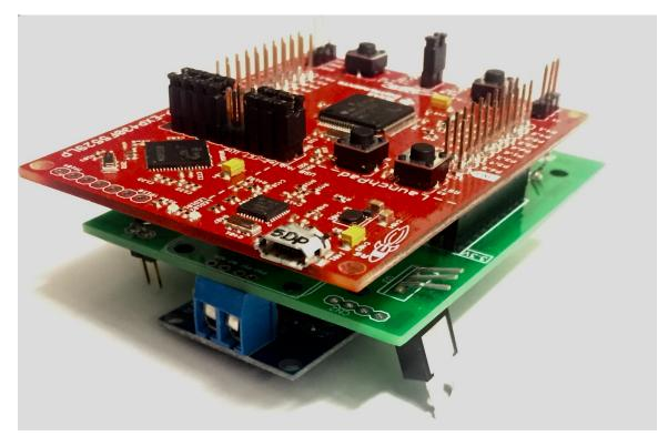
Figure 4.6: MSP430 connected to CAN Shield through the fabricated PCB
