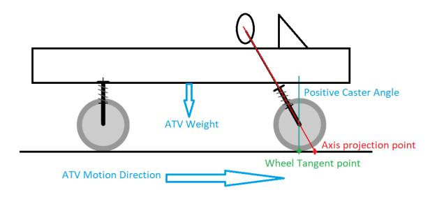
Figure 4.10: Positive Caster Angle for the vehicle direction.
