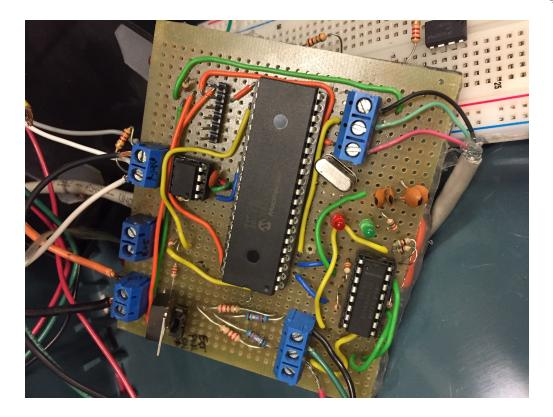
Figure 3.18: Steering Module
