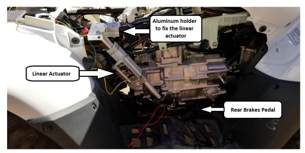
Figure 3.16: Braking System installed on the ATV
