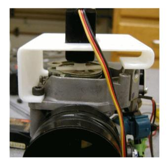
Figure 2.1: Servo attached to the Throttle assembly [9].
