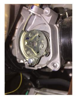
Figure 3.8: Throttle wire and spring at the air valve side.
