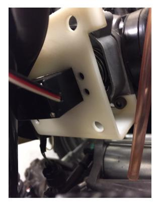
Figure 3.10: Servo Motor attached to fuel pump.
