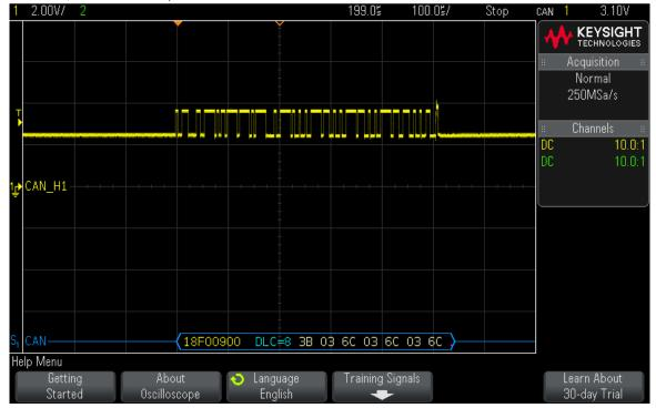
Figure 3.19: CAN message to turn steering right
