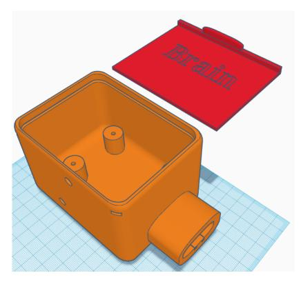
Figure 4.7: The 3D model design for the box used to contain most of the modules
