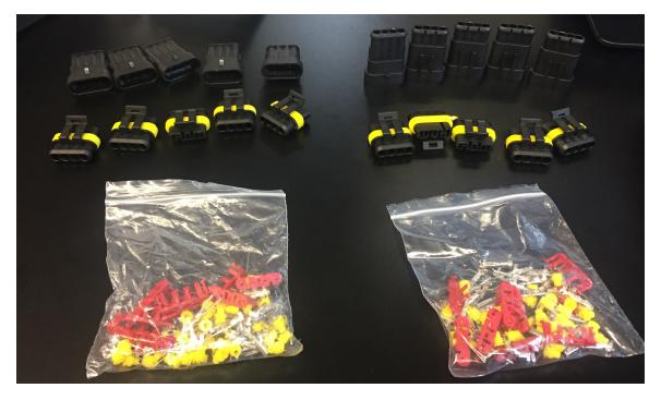
Figure 3.3: CAN Bus Physical implementation: CAN Connectors.
