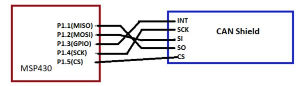
Figure 3.6: MSP430 to CAN Shield Connections.
