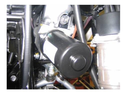
Figure 2.2: DC Power Steering Motor [9].
