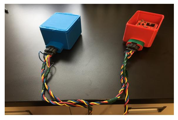
Figure 4.8: The 3D printed boxes connected using CAN bus
