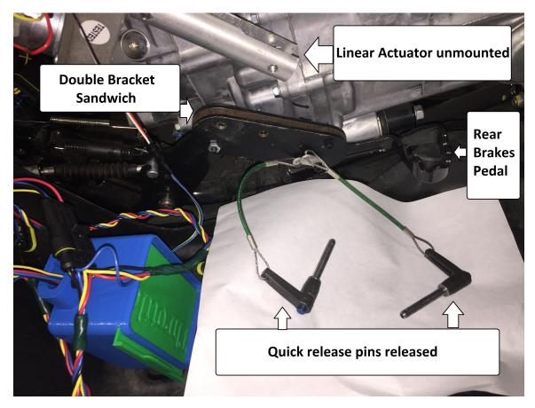
Figure 3.15: Quick release pins released and the braking system unmounted.
