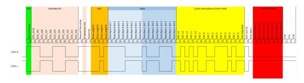
Figure 2.8: Sample of a Standard ID CAN Frame with 2 bytes of data.
