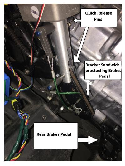
Figure 3.14: Brake Pins fixing the linear actuator to the two-piece bracket sandwiching the brake pedal.
