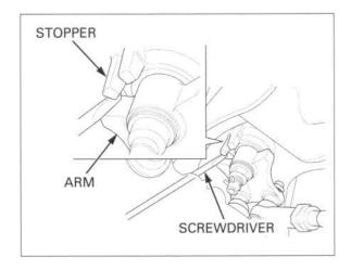
Figure 3.17: Screwdriver position for EPS DTC reset [22].
