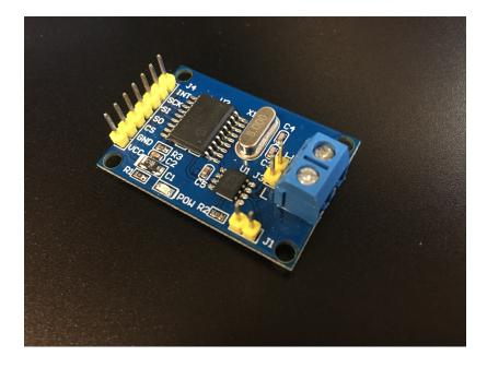
Figure 3.5: The CAN Shield with MCP2515 CAN Transceiver.
