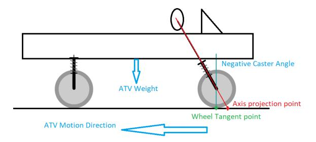
Figure 4.11: Negative Caster Angle for the vehicle direction.
