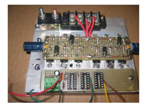
Figure 2.3: H-Bridge circuit attached to large Heat sink [9].
