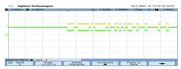
Figure 3.7: CAN Frame on Oscilloscope with Yellow = CAN-H, Green = CAN-L.
