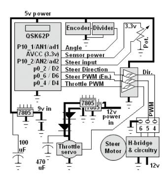
Figure 2.5: Steering circuit using micro-controller to control motor using PWM [8].
