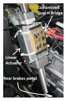
Figure 2.6: Old braking system applied in paper of 2010 [9].
