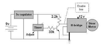
Figure 2.4: Steering PWM test circuit [8].
