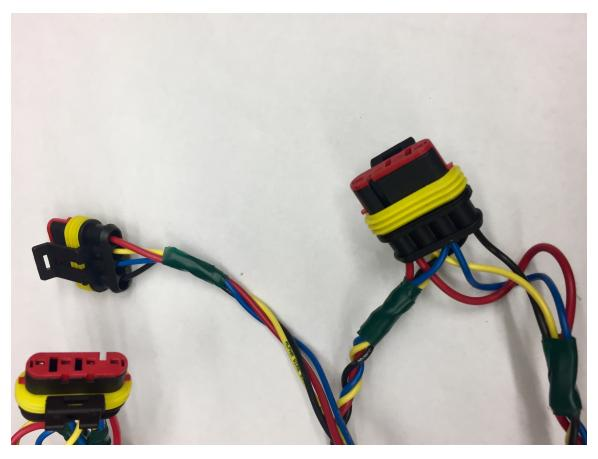
Figure 3.4: CAN Bus Physical implementation: CAN Bus after implementation.
