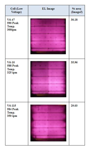
Figure 4.9: Electroluminescence Imaging and ImageJ Calculations [18]
