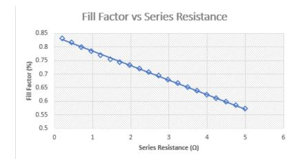
Figure 2.1: Fill Factors vs Series Resistance
