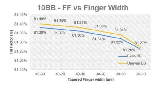
Figure 3.12: 10BB - Fill Factor as a function of TPF width with EBB and UEBB
