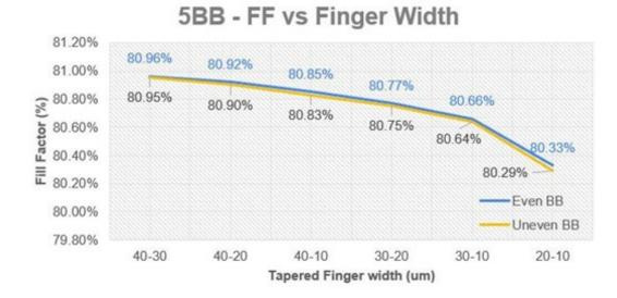
Figure 3.5: 5BB - Fill Factor as a function of TPF width with EBB and UEBB
