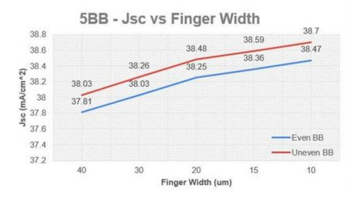
Figure 3.6: 5BB - Short Circuit Current as a function of NTPF width with EBB and UEBB
