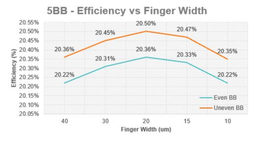
Figure 3.2: 5BB - Efficiency as a function of NTPF width with EBB and UEBB
