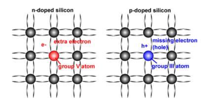
Figure 1.6: Schematic of N-type and P-type semiconductor material [5]
