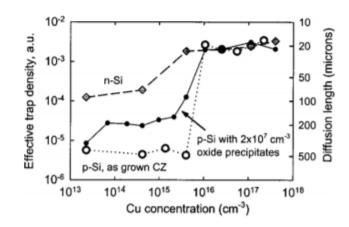
Figure 4.3: "shows 10  $\Omega$ cm CZ grown n-type Si samples (diamonds) effective trap density and minority carrier diffusion length as a function of Cu concentration, CZ grown p-type Si (open circles) at 10 $\Omega$ cm, and internal gettering sites of the order of  $2 \times 10^7 \text{cm}^{-3}$ " [19]
