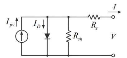
Figure 1.17: Solar Cell Equivalent Circuit
