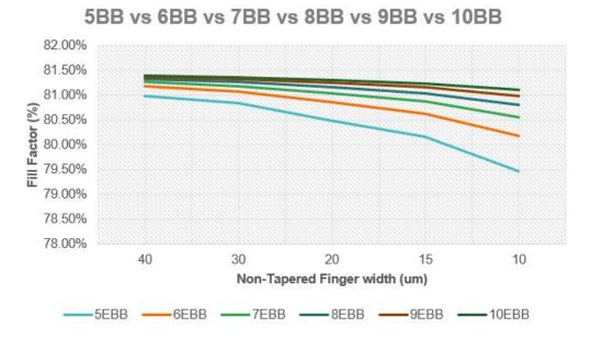
Figure 3.17: 5-10BB - Fill Factor as a function of the NTPF width with EBB
