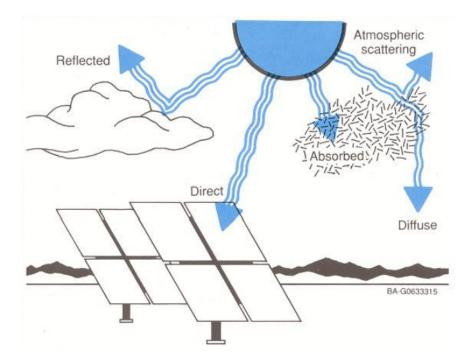
Figure 1.10: Absorption and Scattering of Sunlight by the Earth's Atmosphere [9]
