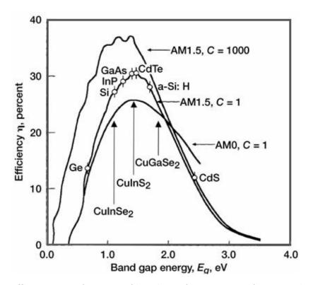
Figure 1.5: Efficiency as a function of band gap for a variety of semiconductor materials [4]
