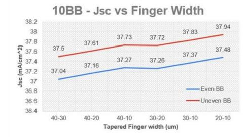
Figure 3.14: 10BB - Short Circuit Current as a function of TPF width with EBB and UEBB
