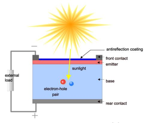
Figure 1.11: Cross-section of a solar cell [10]
