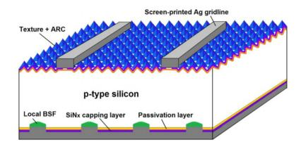
Figure 1.12: PERC Structure [11]
