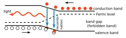
Figure 1.4: Band Diagram of a typical semiconductor [3]
