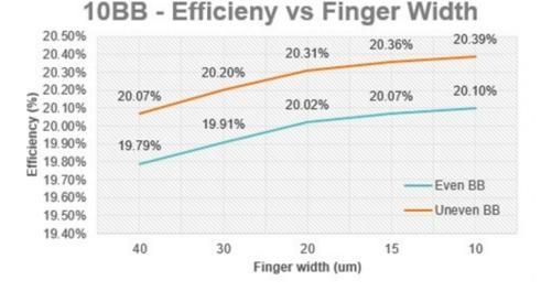
Figure 3.9: 10BB - Efficiency as a function of NTPF width with EBB and UEBB
