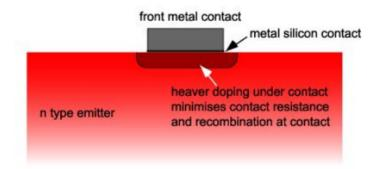
Figure 1.22: High doping of metal contact underside [17]
