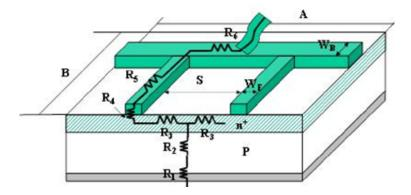
Figure 1.18: Series Resistance Components [15]
