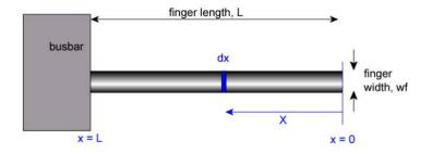
Figure 1.19: Uniform Metal Finger Design [16]
