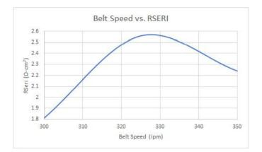
Figure 4.7: Belt Speed vs Series Resistance [18]
