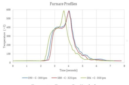
Figure 4.1: Furnace Profiles [18]
