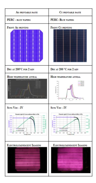
Figure 4.2: Process Sequence for Ag and Cu Pastes, respectively, screen-printed contacts PERC cells [18]
