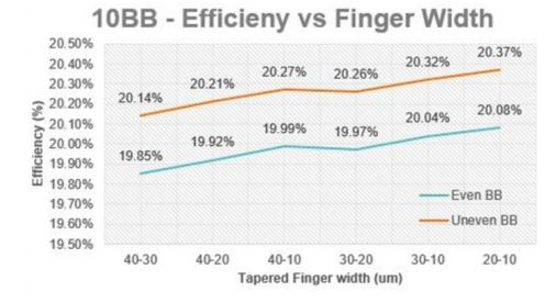
Figure 3.10: 10BB - Efficiency as a function of TPF width with EBB and UEBB
