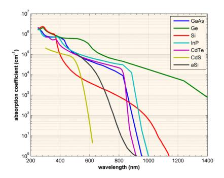
Figure 1.7: "The absorption coefficient,  $\alpha$ , in a variety of semiconductor materials at 300K as a function of the vacuum wavelength of light." [6]
