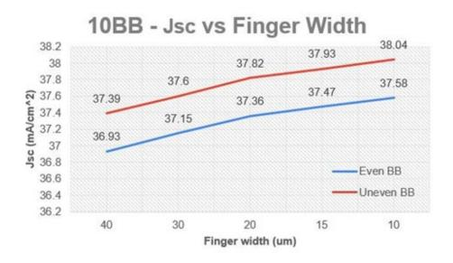
Figure 3.13: 10BB - Short Circuit Current as a function of NTPF width with EBB and UEBB
