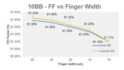
Figure 3.11: 10BB - Fill Factor as a function of NTPF width with EBB and UEBB
