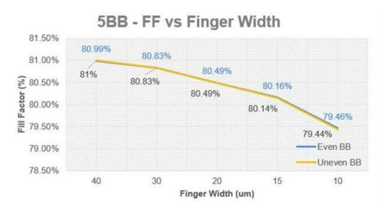
Figure 3.4: 5BB - Fill Factor as a function of NTPF width with EBB and UEBB
