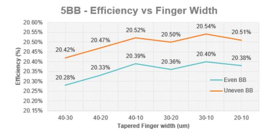
Figure 3.3: 5BB - Efficiency as a function of TPF width with EBB and UEBB.
