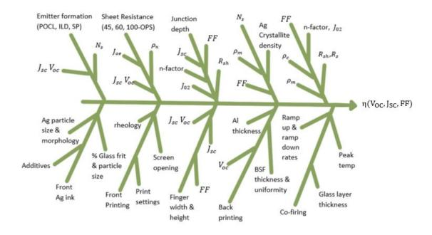
Figure 1.15: Parameters affecting efficiency [14]
