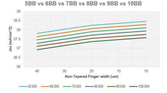
Figure 3.18: 5-10BB - Short Circuit Current as a function of the NTPF width with EBB
