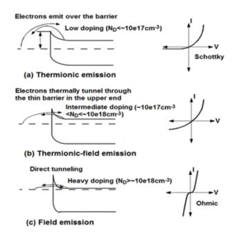
Figure 1.20: Conduction mechanism for metal-semiconductor contacts [14]
