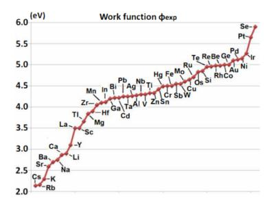
Figure 1.21: Work functions of a variety of elements [14]
