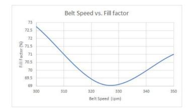
Figure 4.8: Belt Speed vs Fill Factor [18]
