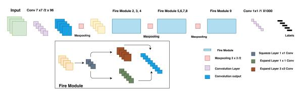
Figure 2.2: SqueezeNet architecture
