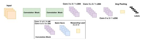
Figure 2.3: Alexnet architecture
