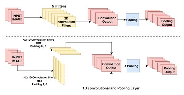
Figure 4.1: Implementation of 1D CNN replacement layer
