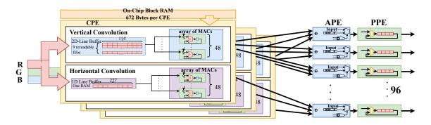
Figure 4.4: complete 1D replacement layer hardware architecture
