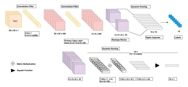
Figure 2.4: Capsnet Architecture
