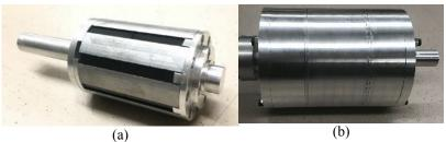
Figure 3-9. (a) High-speed inner rotor assembly (b) fullly assembled MG
