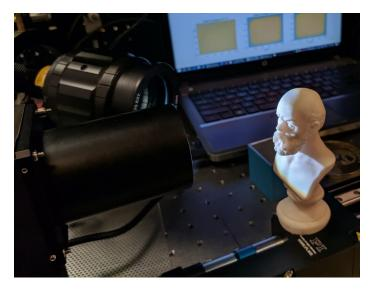
Figure 4.21: Apparatus setup for experiment 5 with the modified GP-SIDH system under reflective illumination.
