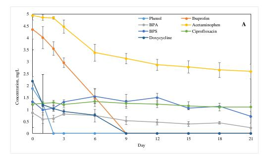
Figure 18. Contaminants removal in fungal batch reactors(mean±SD); Biotic(A), abiotic with fungal mass (B), abiotic without fungal mass (C)
