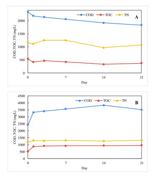
Figure 26. Aggregate parameters in fungal batch reactors for mixed cell leachate; Biotic(A), abiotic with fungal mass (B), abiotic without fungal mass (C)
