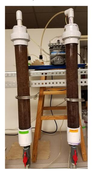
Figure 3. Plug flow column reactors (Left, biotic and right, abiotic)
