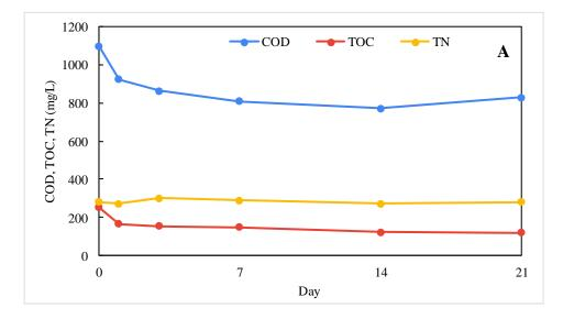
Figure 23. Aggregate parameters in fungal batch reactors for S1 leachate; Biotic(A), abiotic with fungal mass (B), abiotic without fungal mass (C)
