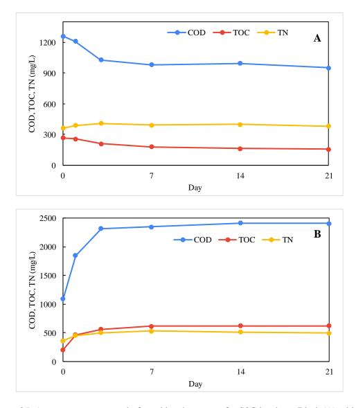
Figure 25. Aggregate parameters in fungal batch reactors for S2C leachate; Biotic(A), abiotic with fungal mass (B), abiotic without fungal mass (C)
