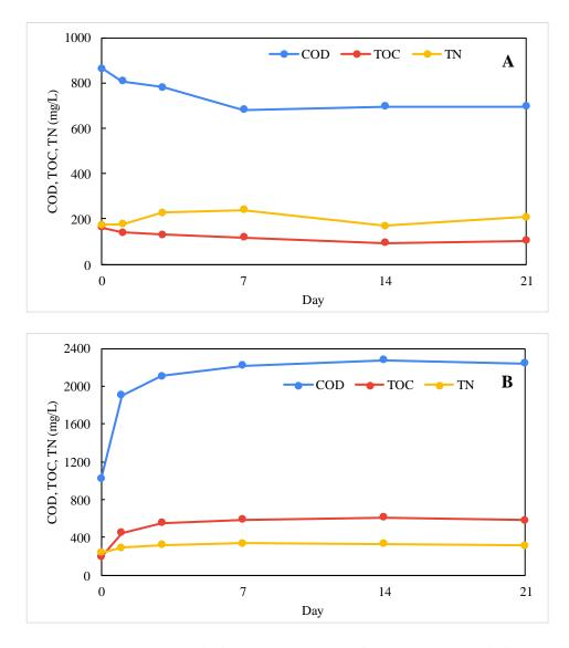
Figure 24. Aggregate parameters in fungal batch reactors for S2A leachate; Biotic(A), abiotic with fungal mass (B), abiotic without fungal mass (C)
