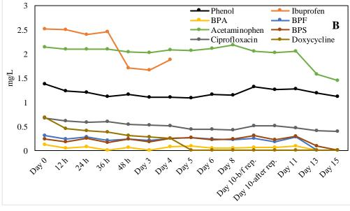
Figure 40. Contaminants removal in fungal plug flow reactors; Biotic(A), abiotic with fungal mass (B)
