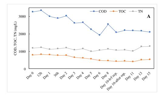
Figure 39. Aggregate parameters in fungal column reactors; Biotic (A), abiotic with fungal mass (B)
