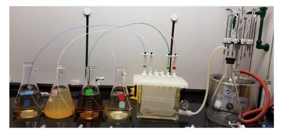
Figure 2. Loading of LL samples on SPE cartridges
