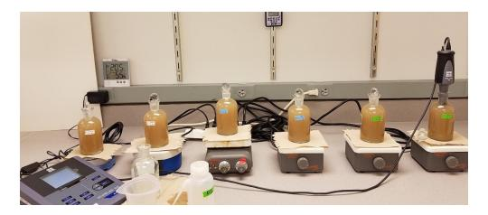
Figure 4. AS respiration inhibition test
