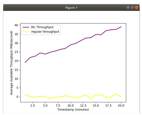
(a) Target Link Throughput over time. ML Model Added Intelligence vs. Original Topology with no additional Intelligence
