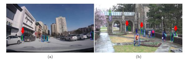
Figure 3.8: The impact of accuracy reduction on video frame modification by the latency controller for JAAD (a) and DukeMTMC (b). Green and blue bounding boxes indicate pedestrian detections on unmodified and modified video frames respectively. The video frames experience an accuracy loss of  $\approx 3\%$  for JAAD and  $\approx 4\%$  for DukeMTMC respectively. The red arrows show the resulting detection errors.
