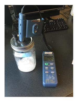
Figure 3. Relative humidity jar and measurement device
