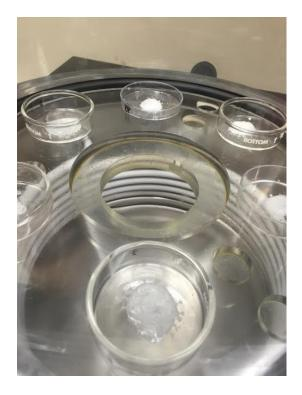
Figure 5. TCH samples in the evaporative dryer
